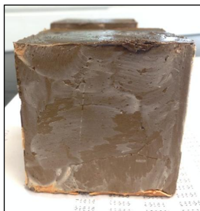
Figure 25: Physical Characteristics of Fly-ash based Geopolymer Cement with 10 M NaOH (Formulation 1) After Immerse in Sulfuric Acid at 0.2 M.
