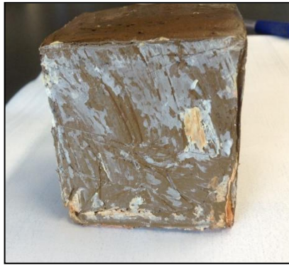
Figure 27: Physical Characteristics of Fly-ash based Geopolymer Cement with 15 M NaOH (Formulation 1) After Immerse in Sulfuric Acid at 0.2 M.
