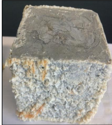
Figure 21: Physical Characteristics of Class G Cement After Immerse in Sulfuric Acid at 0.2 M.
