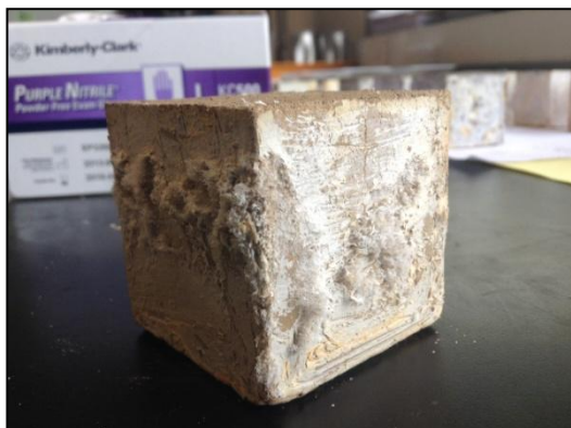
Figure 24: Physical Characteristics of Fly-ash based Geopolymer Cement with 12 M NaOH (Formulation 1), After Immerse in Sulfuric Acid at 1 M.
