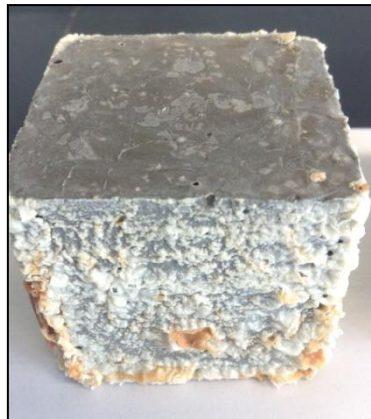
Figure 22: Physical Characteristics of Class G Cement After Immerse in Sulfuric Acid at 1 M.
