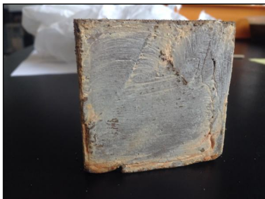
Figure 23: Physical Characteristics of Fly-ash based Geopolymer Cement with 12 M NaOH (Formulation 1) After Immerse in Sulfuric Acid at 0.2 M.
