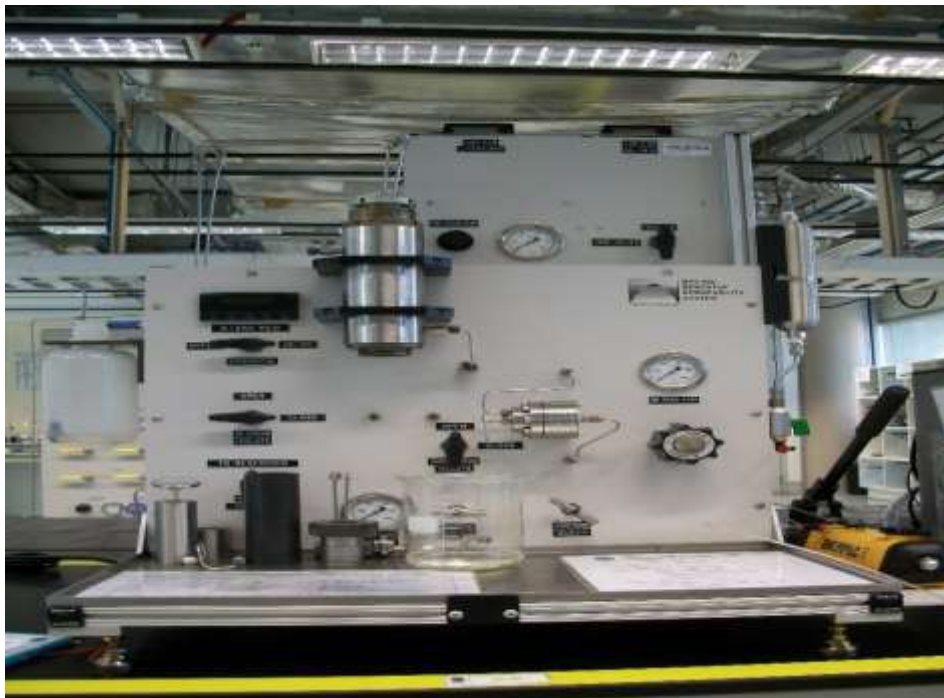
Figure 13: Benchtop permeability system setup
