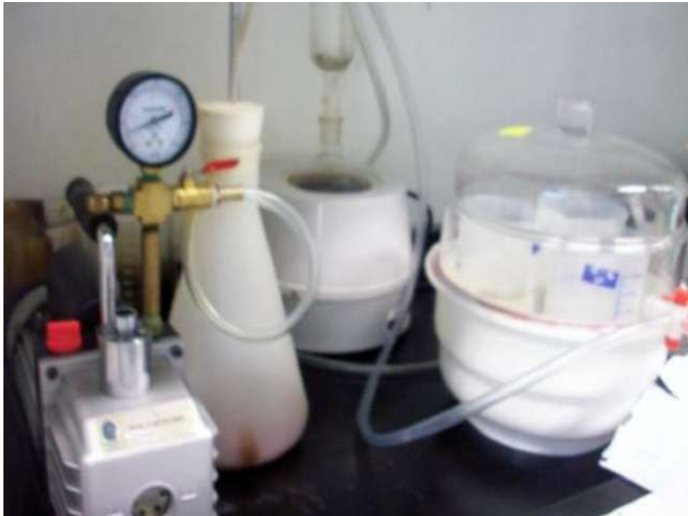
Figure 12:Desiccators with positive displacement pump setup
