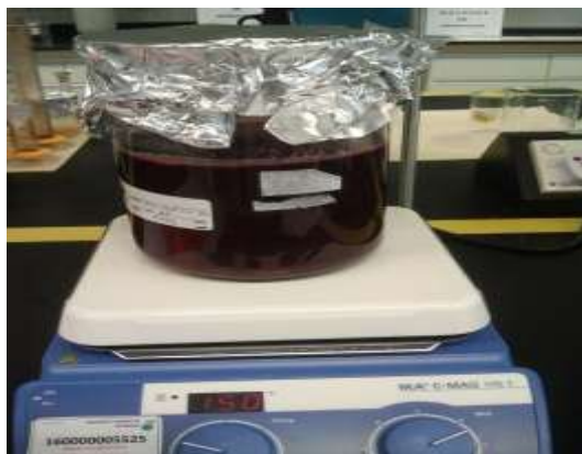
Figure 7: Cooking CR with NaOH at 150°C
