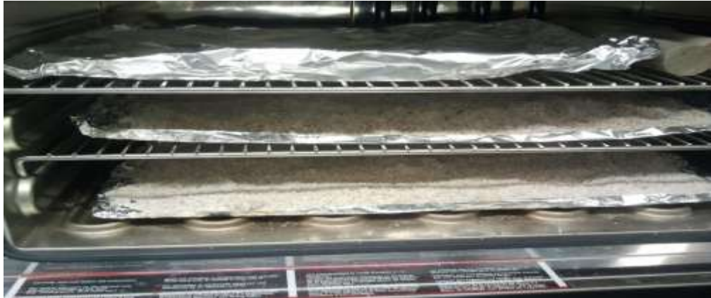
Figure 5: Drying process of CR in oven at 50° C for 2 days.
