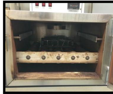
5) Cure the cement slurry in the oven at 60°C for 24 hours
