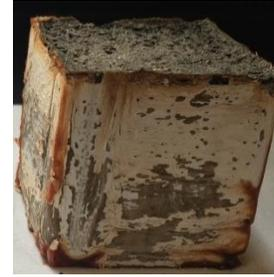
Figure 13: Cement cube by using 300µM MIRHA
