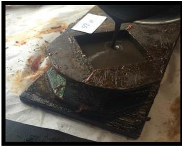
4) Pour the slurry into the mold
