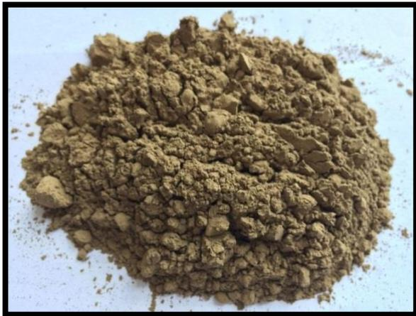
Fly Ash (ASTM Class F)
