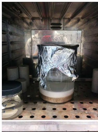
Figure 10: Coconut husk alkali-based reaction with chloroacetic acid
