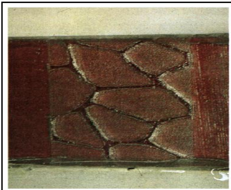
Figure 51 : Fracture network and matrix micromodel with ceramic boundaries sample constructed in Zhang research
