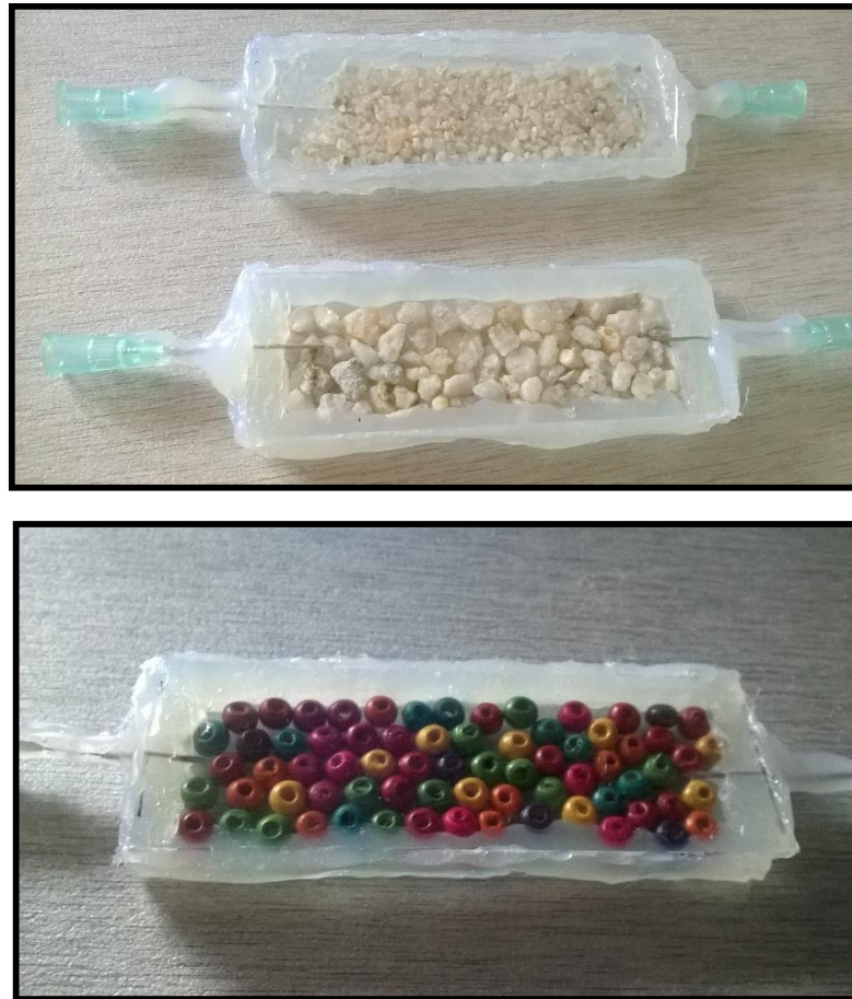
Figure 24 : Micromodel with small size grains (above), micromodel with medium size grains (middle), and micromodel with large size grains (bottom)
