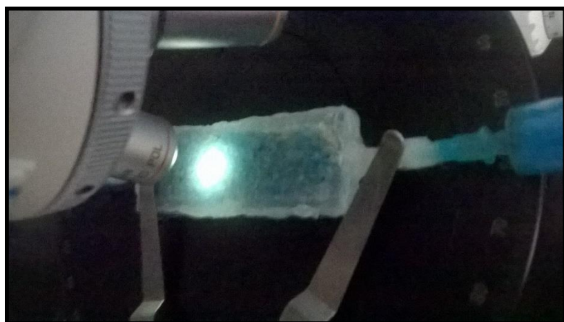
Figure 22 : Syringe containing dyed-water (blue) was connected to the inlet port of micromodel
