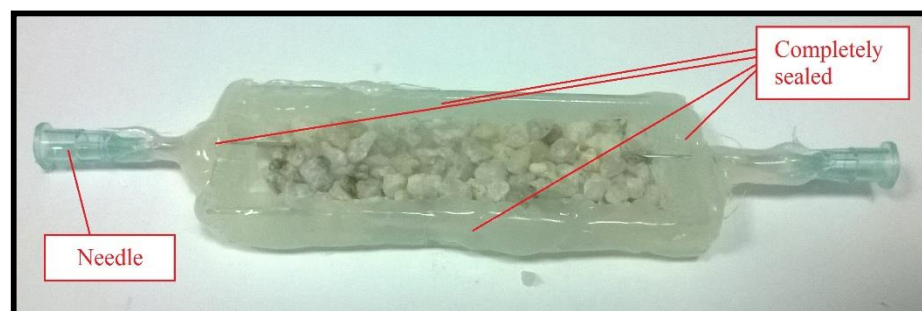
Figure 12 : After the sand compaction and being sealed completely
