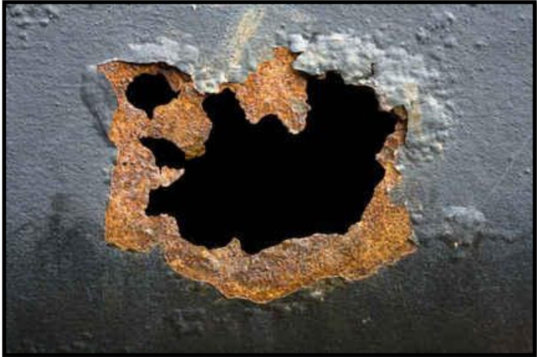
**Figure 5: Leak due to Pitting Corrosion in a pipe line**
