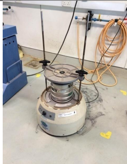
Figure 14: Sand screening machine
