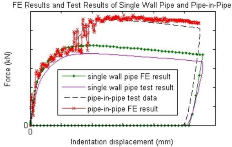
Figure 7: Comparison between test result and FE result (Zheng, et, al. 2012)
