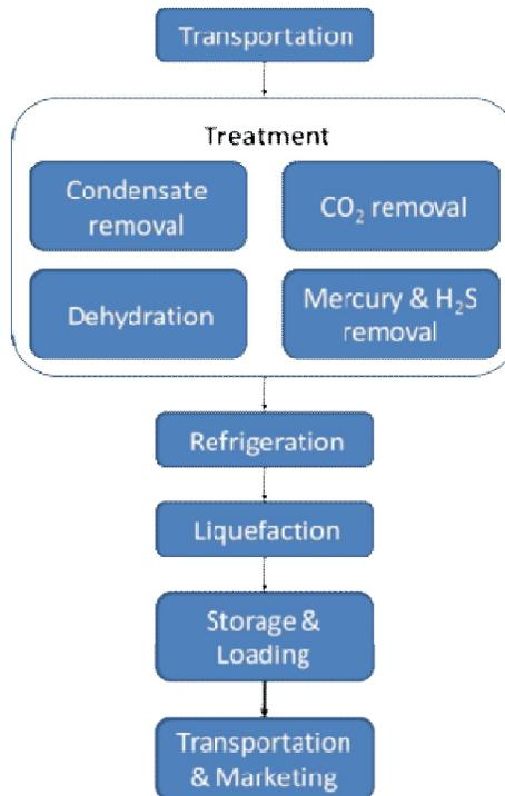
Figure 1: A typical LNG Process
