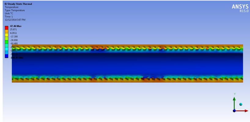
Figure 24: Temperature distribution of Invar pipe
