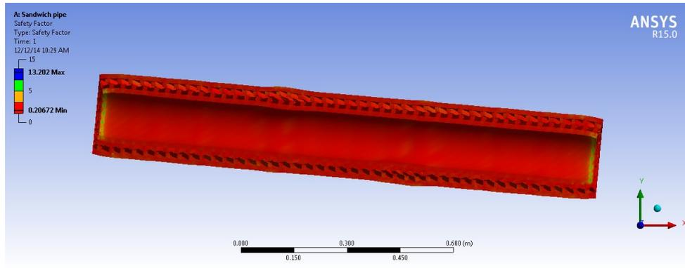
Figure 17: Safety factor distribution of SS 304L pipe
