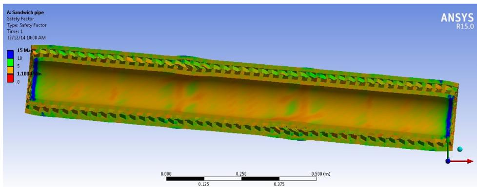
Figure 21: Safety factor distribution of Kovar pipe
