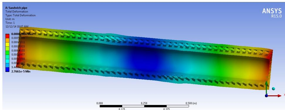
Figure 18: Total deformation of Kovar pipe
