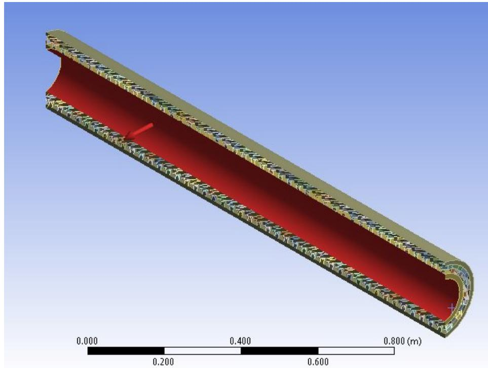
Figure 11: Applied internal pressure load
