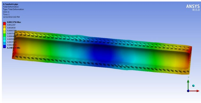
Figure 22: Total deformation of Invar pipe
