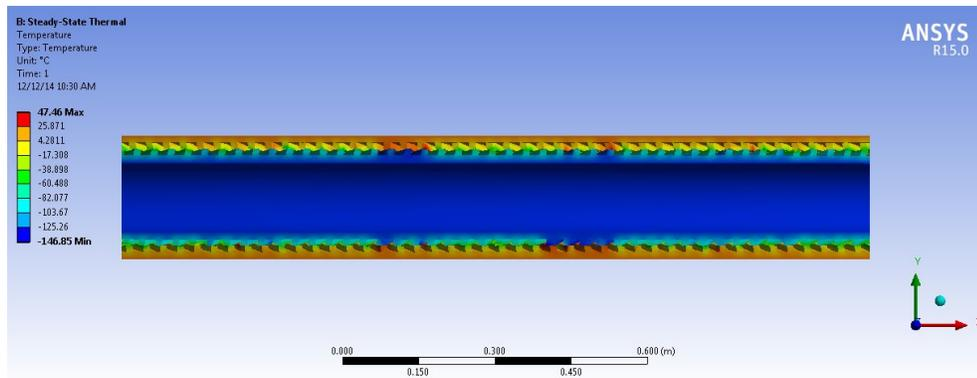
Figure 16: Temperature distribution of SS 304L pipe
