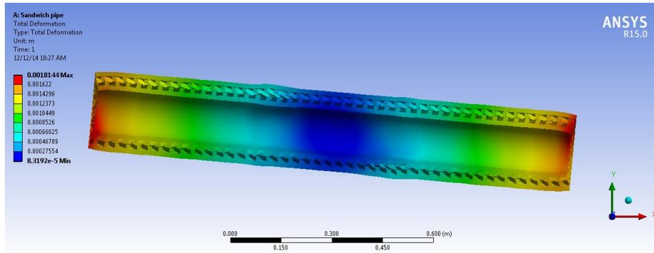
Figure 14: Total deformation of SS 304L pipe
