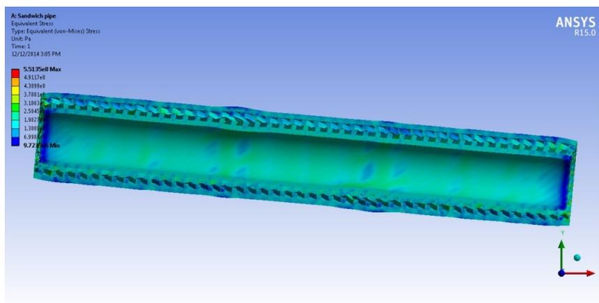
Figure 23: Stress distribution of Invar pipe
