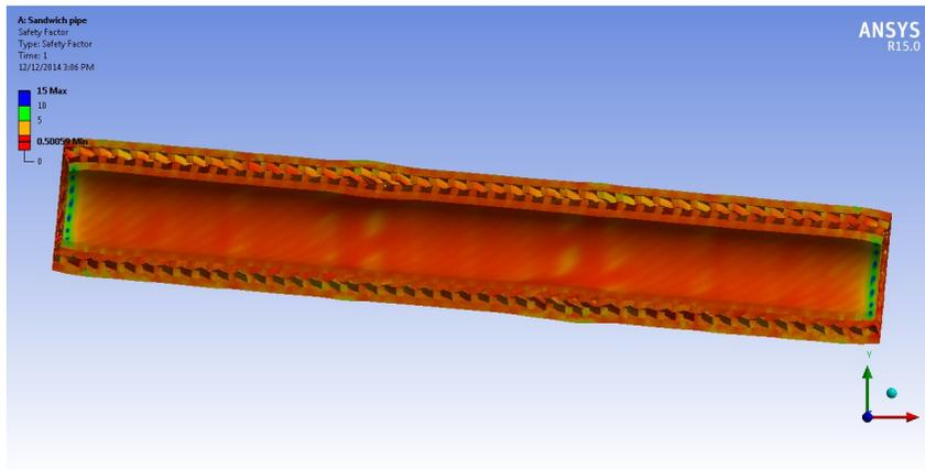
Figure 25: Safety factor distribution of Invar pipe
