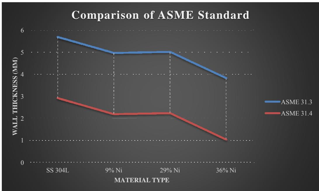
Figure 26: Comparison of ASME standards
