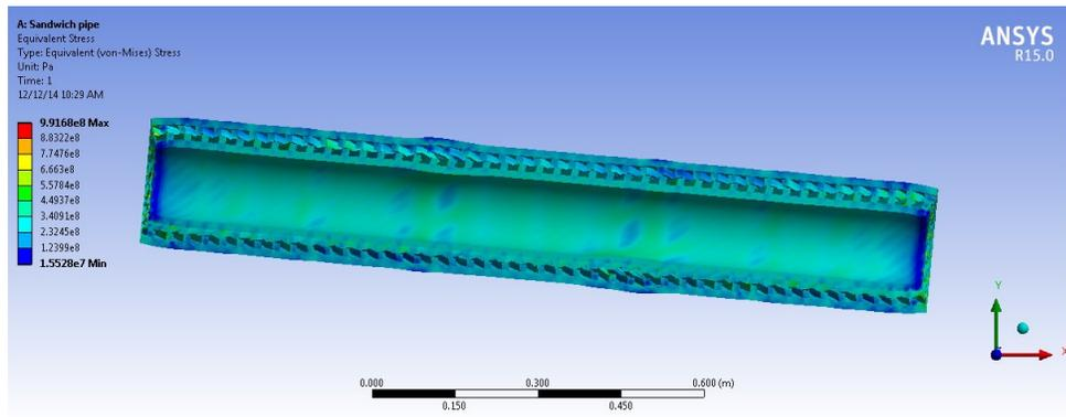
Figure 15: Stress distribution of SS 304L pipe
