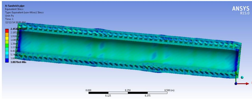
Figure 19: Total stress distribution of Kovar pipe
