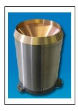
Figure 5: Rain gauge (Tipping Bucket)[7]
