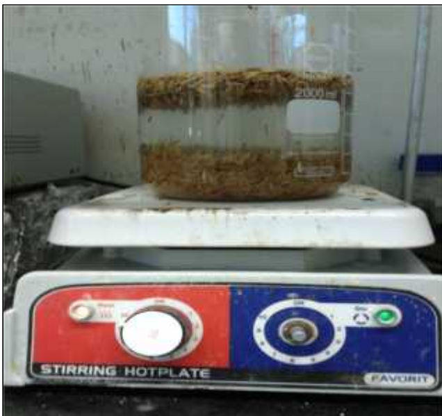
Figure 9: rice husk mix with hydrochloric acid (HCl) on the top surface of hot plate.
