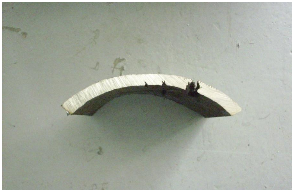
Figure 4.6: Penetrated internal crack
