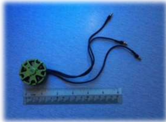
Figure 15: BLDC outrunner motor
