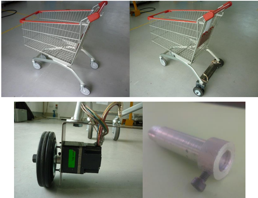
Figure 19: Modifying Shopping Cart's Wheels
