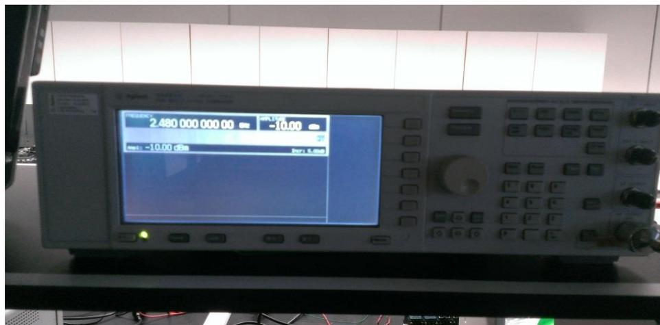
Figure 3.7: Input signal from RF Signal Generator with -10dBm.
