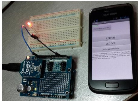
Figure 18: Testing BlueBee and XBee Shield with Android
