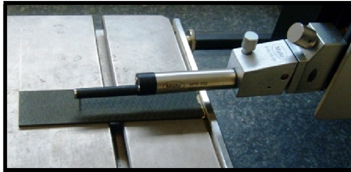
Figure 11: Surface Roughness of the Sample Is Measured Using Perthometer
