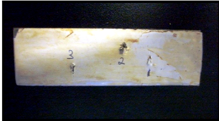
Figure 27: Scratch Test Done On Random Location
