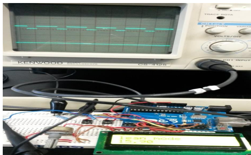
Figure 12: The PWM output voltage and the filtered DC output voltage from the RC circuit signals for Lean mode 2 using the oscilloscope
