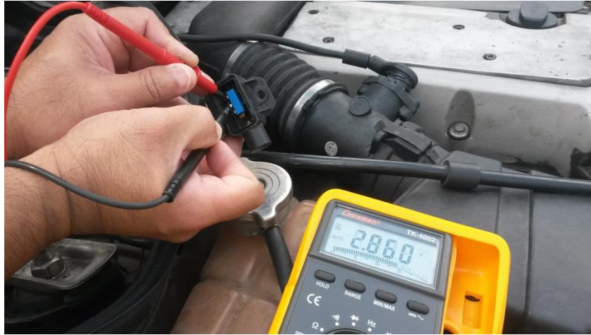
Figure 11: Maximum output voltage from the CO potentiometer while the engine is running
