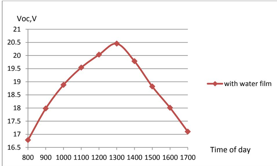
**Figure 35:Solar panel with water film on 4 November**
