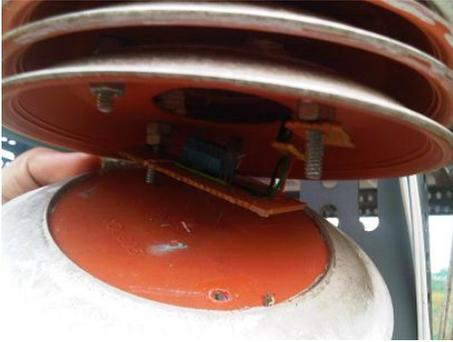
**Figure 10: ambient temperature and humidity sensor**
