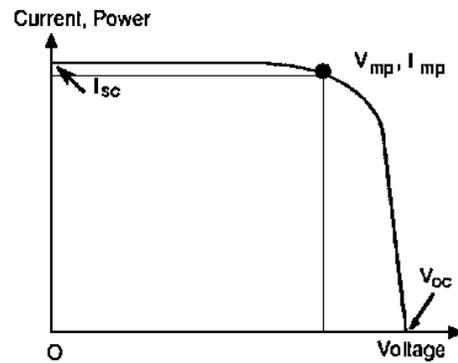
Figure 20: I<sub>sc</sub> VS V<sub>oc</sub> graph
