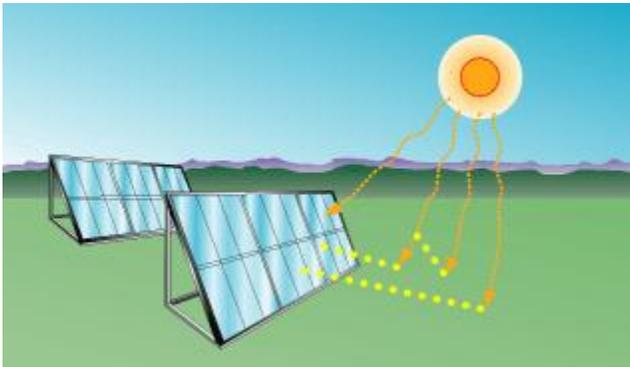
*Flat-plate collectors, which typically contain a large number of solar cells mounted on a rigid, flat surface, can make use of both direct sunlight and the diffuse sunlight reflected from clouds, the ground, and nearby objects*
