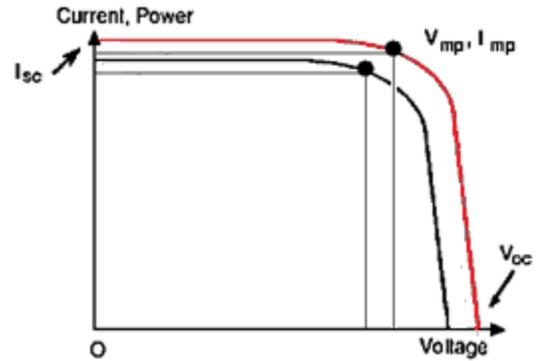
Figure 21:  $I_{sc}$  VS  $V_{oc}$  graph [7]. Figure 22: Increase of  $V_{mp}$  and  $I_{mp}$  when  $V_{oc}$  increases [7].
