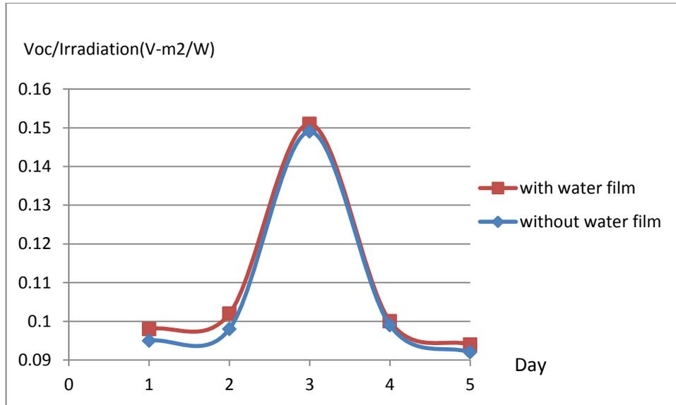
**Figure 38: Comparison graph of average  $V_{OC}/Irradiation$  for solar panel with and without water film per day.**
