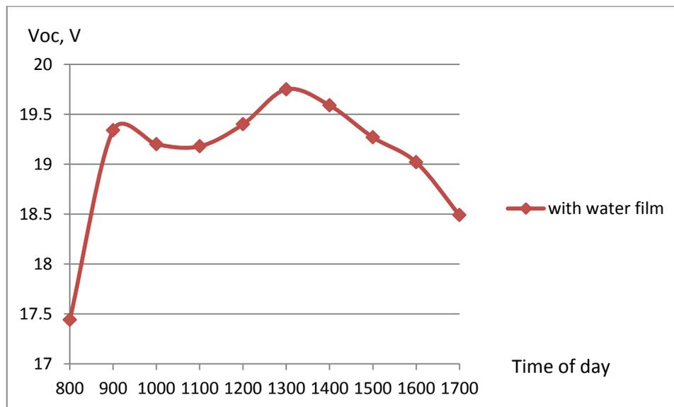
**Figure 29: Solar panel with water film on 2 November**
