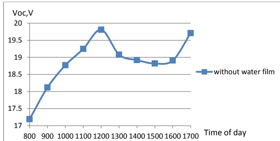
**Figure 24: Solar panel without water film on 30 October 2010**
