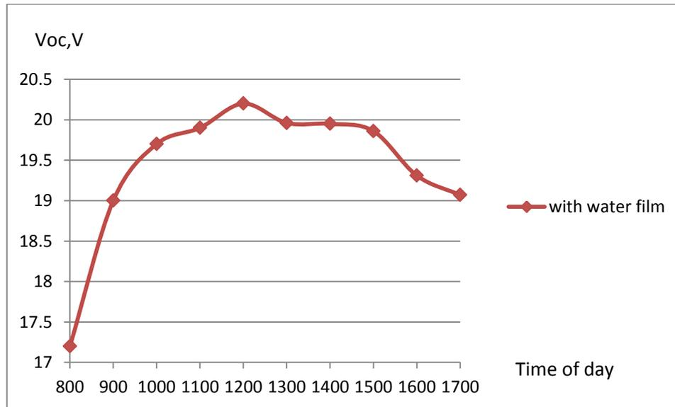
**Figure 26: Solar panel with water film on 1 November**
