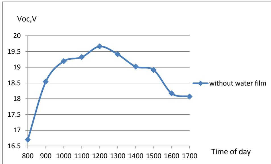
**Figure 27: Solar panel without water film on 1 November**
