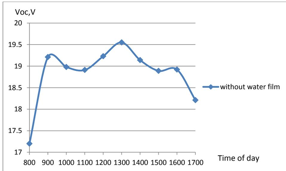
**Figure 30: Solar panel without water film**
