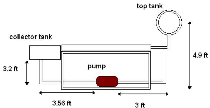
Figure 40: Solar stand pump sizing
