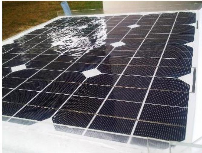
**Figure 17: Creation of water film from overflowing the dam**
