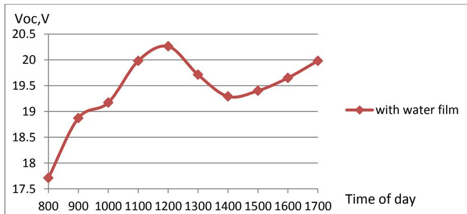
Figure 23: Solar panel with water film on 30 October 2010
