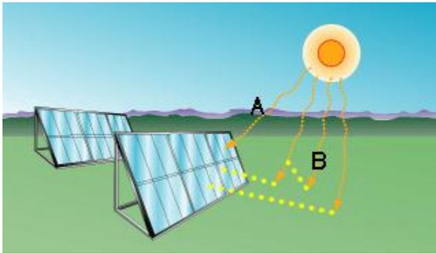
*Diffuse sunlight (B), reflected from clouds, the ground, and nearby objects, and direct sunlight (A) falling onto flat-plate solar panel*
