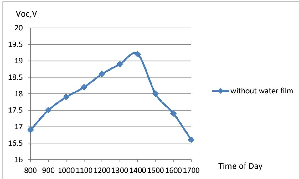
**Figure 33: Solar panel without water film on 3 November**
