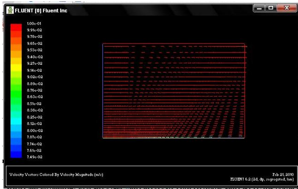
Figure 11: Boundary Layer Profile
