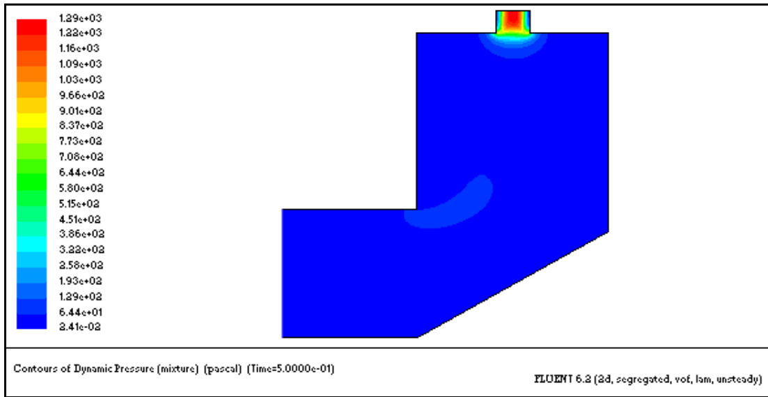
Figure 35: Contours of dynamic pressure (mixture) of Design3 (0.5s flow)
