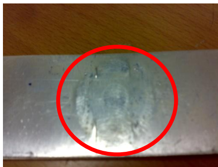
Figure 4.18: 'ring' shape behind welding sample
