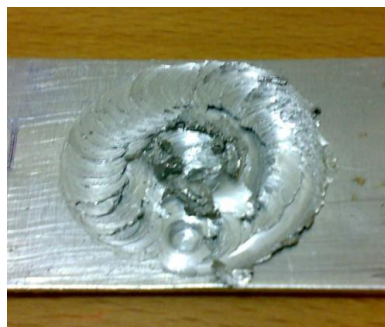
Figure 4.7: Formation of the welding (penetration 1.5mm)
