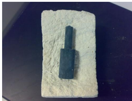
Figure 4.4: The tool after undergone the heat treatment
