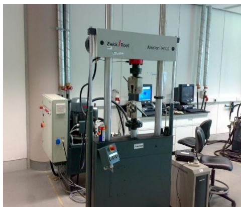
Figure 4.10: Lap shear test using Universal Testing Machine
