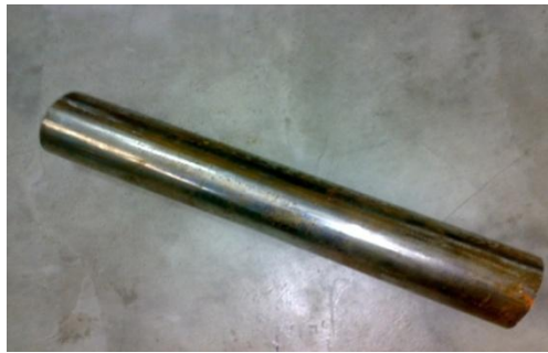
Figure 3.2: the raw material for the tool: AISI H13
