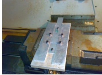
Clamp the jig inside the machine
