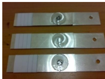
Figure 4.9: sample of the swept FSSW welded plate
