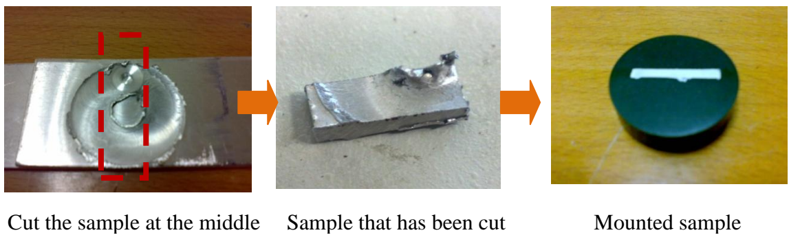
Figure 4.15: Preparation of the sample for mounting process
