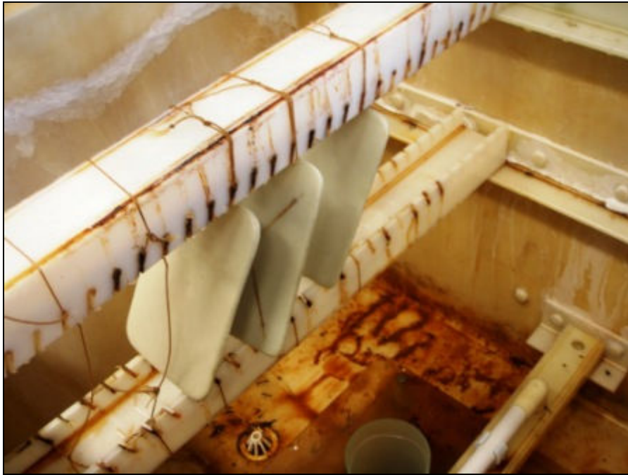
Figure 5: Polyurea specimens in salt spray chamber
