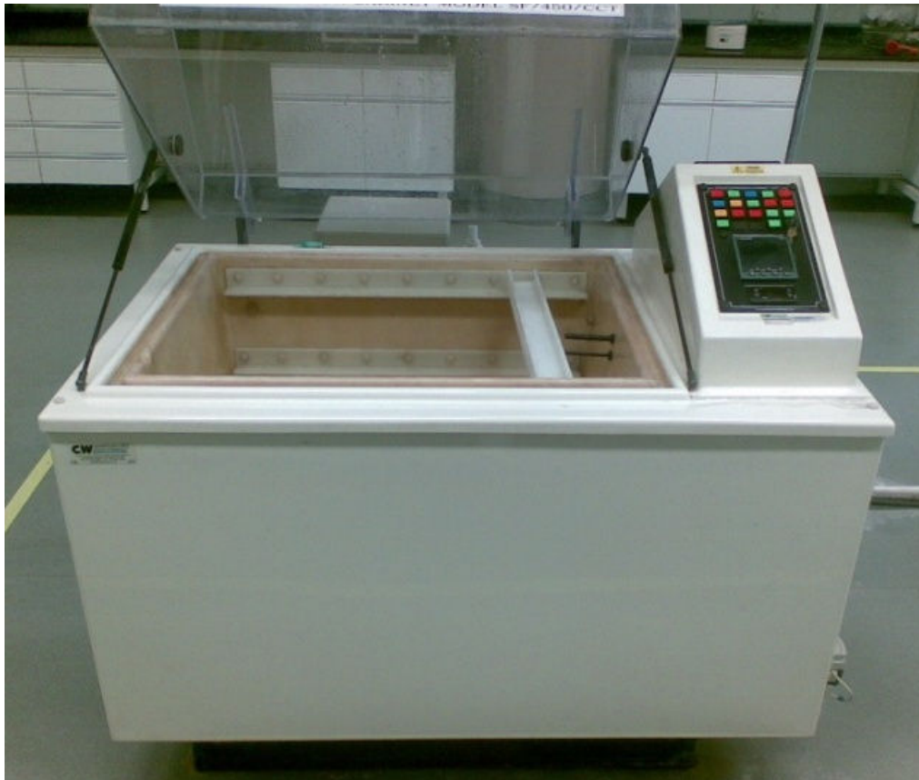
Figure 4 : “Cyclic Corrosion Cabinet (CCT)” model: SF/450 CCT
