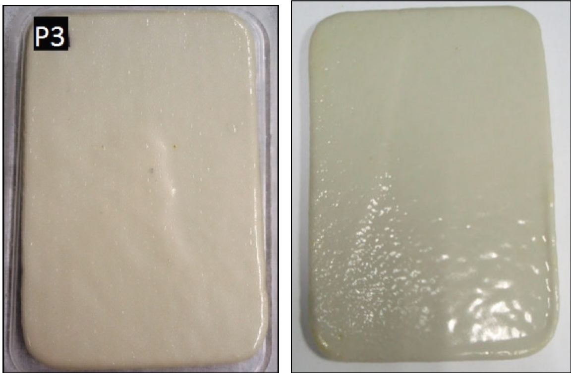
Figure 13: Specimen P3-U – primary face (left) & reverse face (right)
