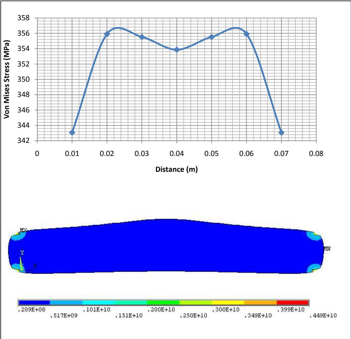
Figure 10: Von Mises stress distribution
