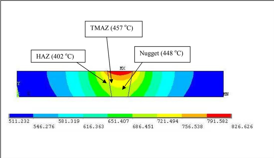
Figure 9: Temperatures in different zones of the FSW
