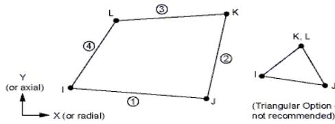
**Figure 4: PLANE182 geometry**
