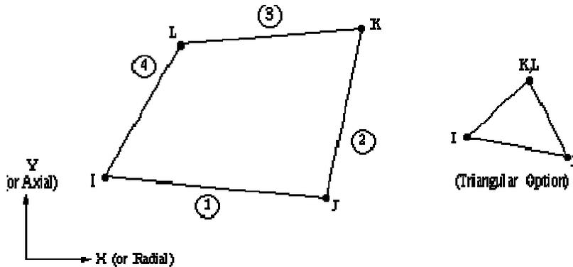
**Figure 3: PLANE55 Geometry**
