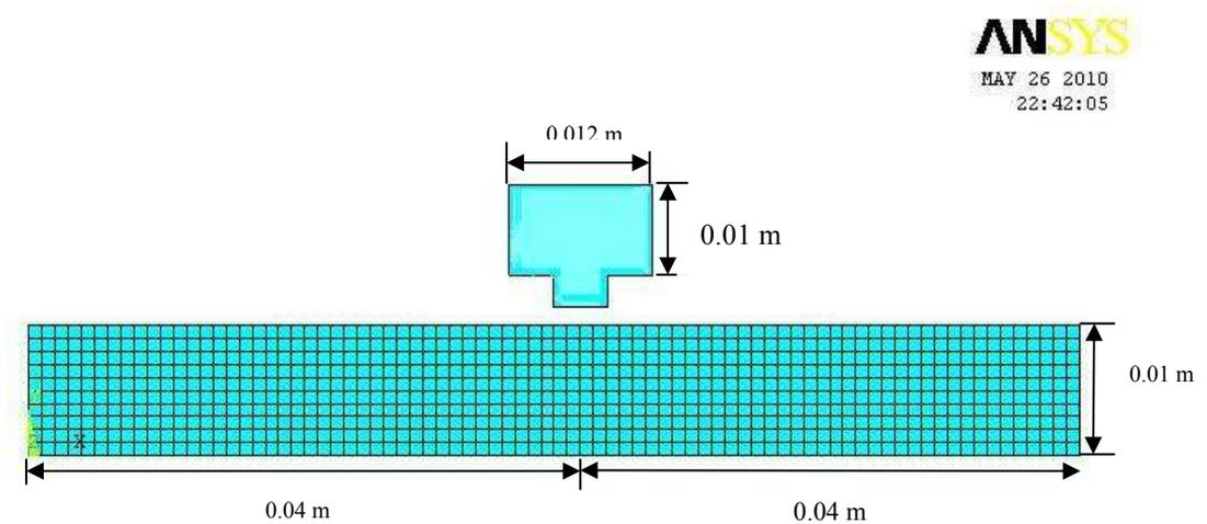
**Figure 5:** Meshed model of work piece
