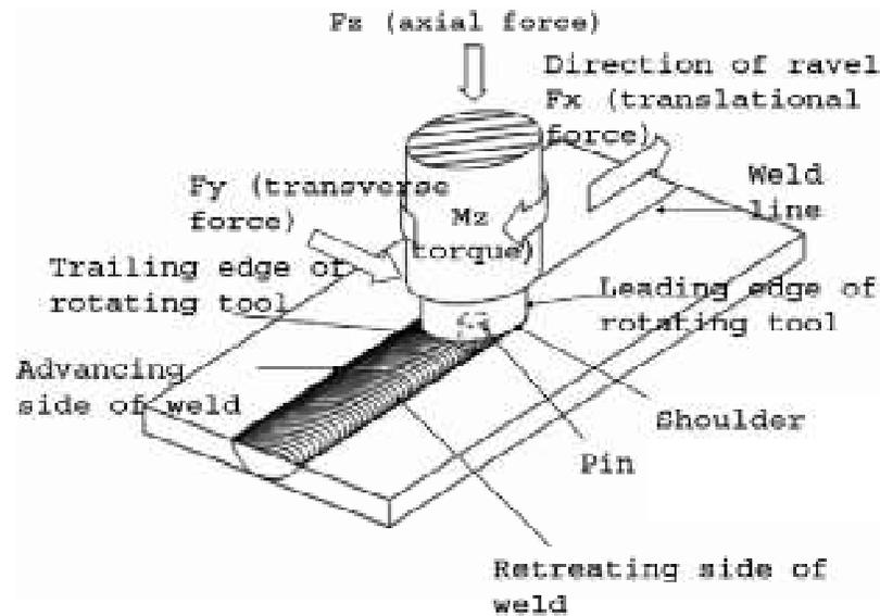
**Figure 1:** Schematic drawing of the friction stir welding [4]
