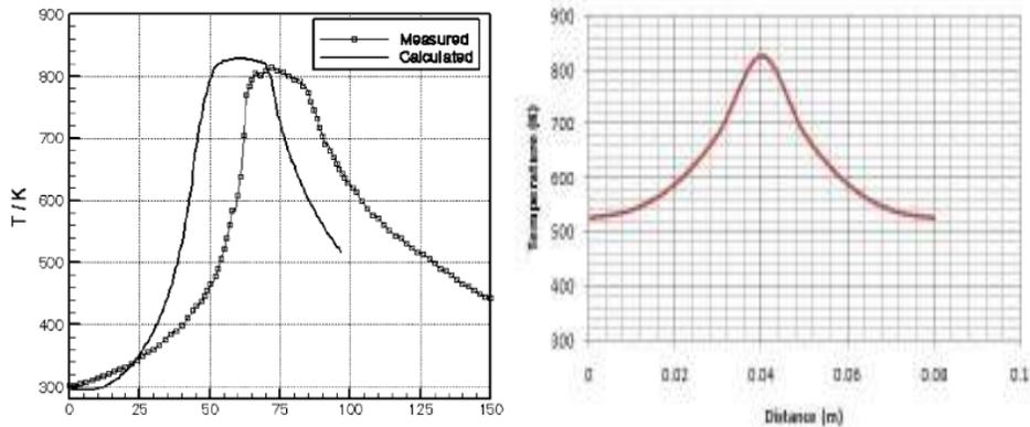
**Figure 7:** Comparison of temperature distribution produced with Song and Kovacevic [12] model
