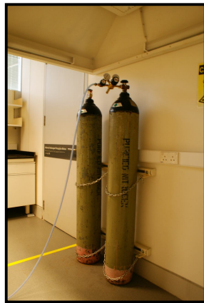
Fig.3.5: Nitrogen tank (supply nitrogen)
