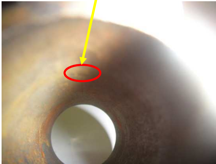
Figure 4-3 : The sample after drop test (height = 100cm)
