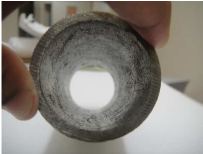
Figure 4-1 : The sample after drop test (height = 20cm)
