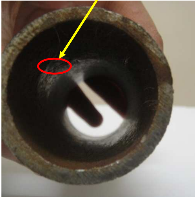
Figure 4-4 : The sample after drop test (height = 140cm)
