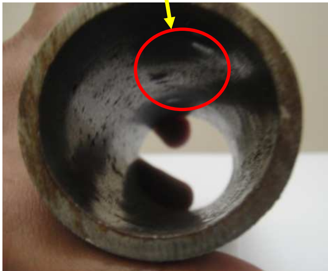
Figure 4-5 : The sample after drop test (height = 180cm)
