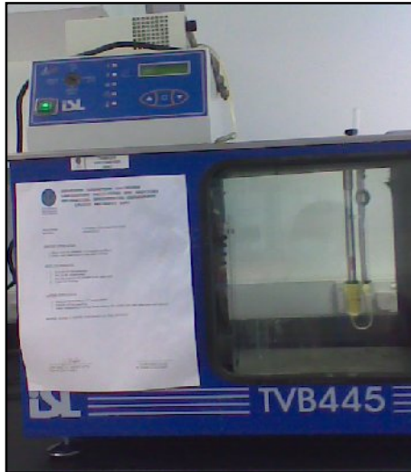
Figure 3.5: The TAMSON Viscometer unit (Inside it, Ubbelohde viscometer)
