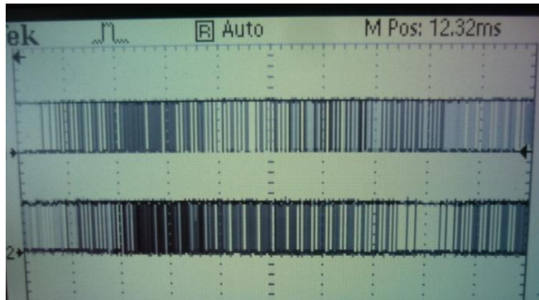
Figure 27: SPWM signals (phase 1 and phase 2) at output frequency of 45 Hz
