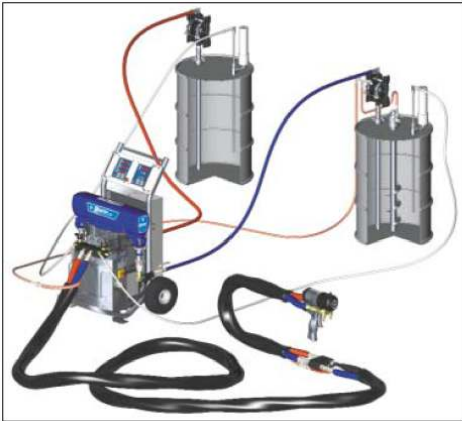
Figure 5: High pressure polyurea equipment
