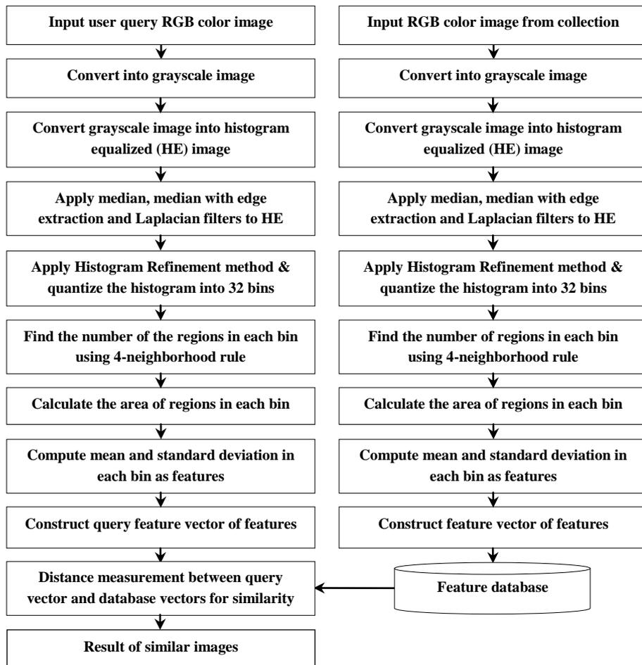
Figure 3.5 Step wise block diagram of the proposed Approach-2.
