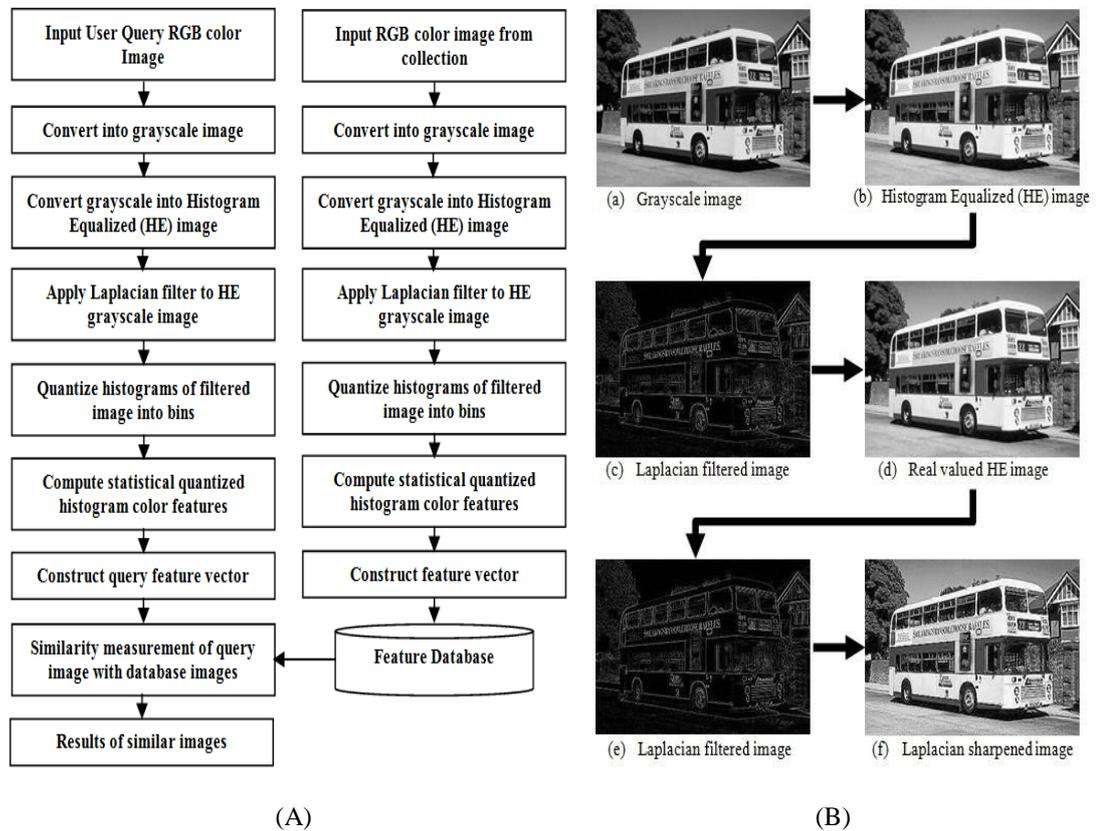
**Figure 3.2** (A) Block diagram of the proposed Approach-1 (B) Sharpening process using Laplacian filter.
