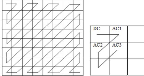
**Figure 3.12** Selection of  $8 \times 8$  DCT block coefficients in zigzag order.
