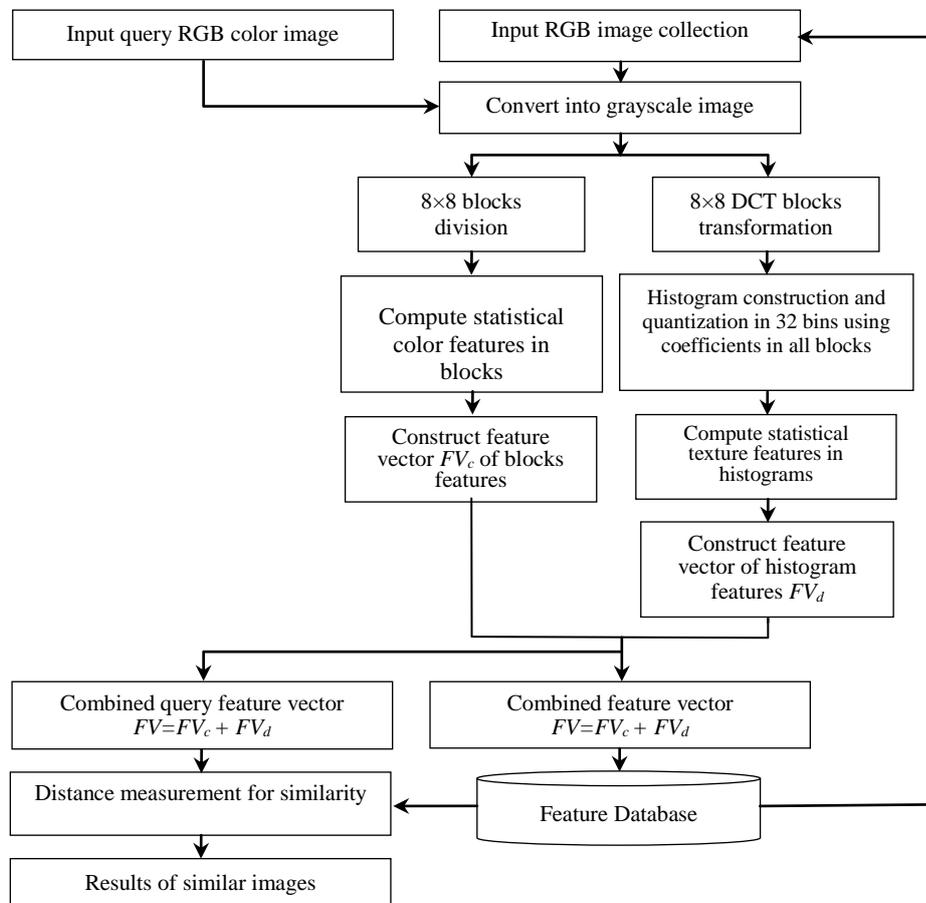
**Figure 3.15** Block diagram of the proposed Approach-10 based on the combination of the color and texture features in the spatial and frequency domains.
