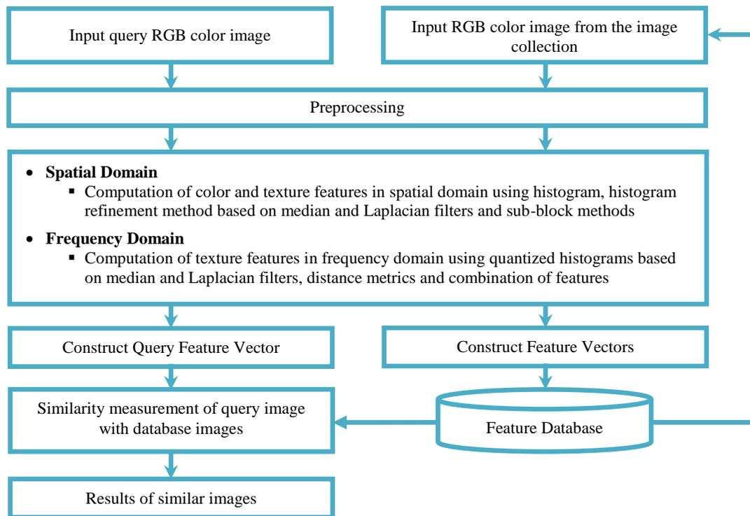
**Figure 3.1** Overview of the entire CBIR using hybrid methods with color and textures features in the proposed approaches in the spatial and frequency domains.
