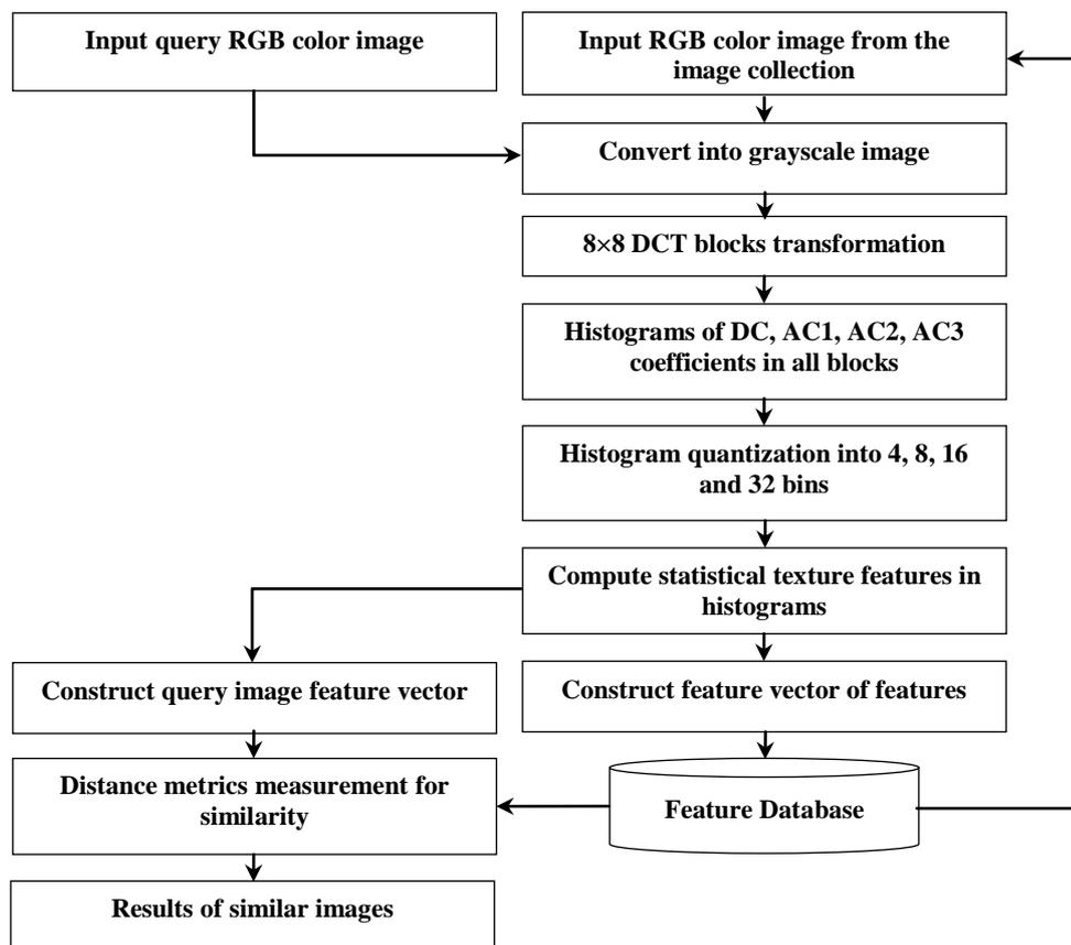
**Figure 3.13** Step wise block diagram of the proposed Approach-7.
