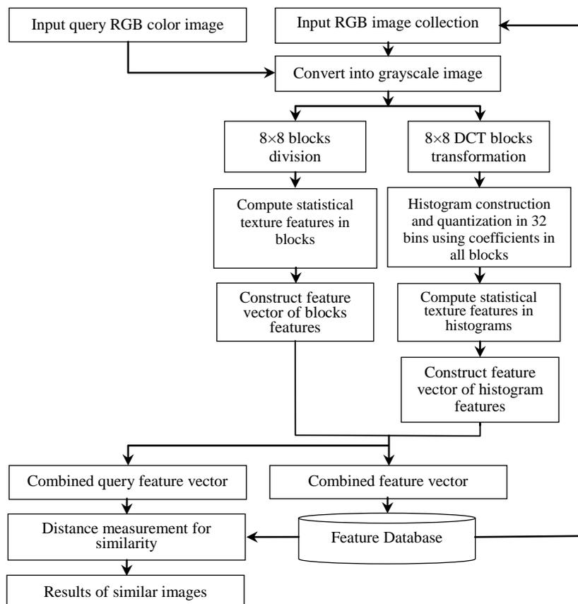
**Figure 3.14** Block diagram of the proposed Approach-9 based on the combination of the texture features in the spatial and frequency domains.
