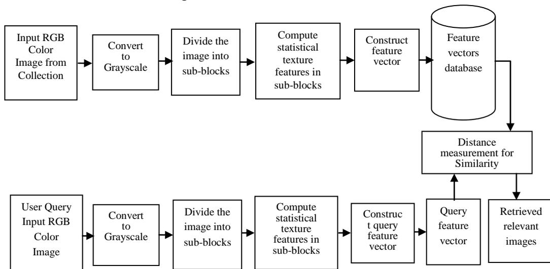
**Figure 3.8** Block diagram of the proposed Approach-4.
