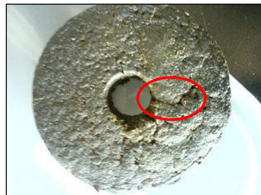
Sample B – Crack found , 11mm in length
