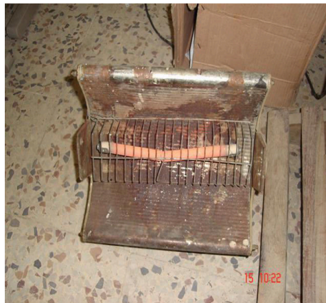
Figure 2.34: Unsafe Electric Heaters being used at PFSs.
