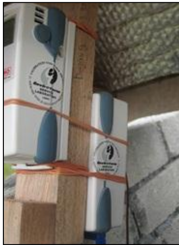
Figure 3.17: Position of hygro-thermometers inside house model (side view)
