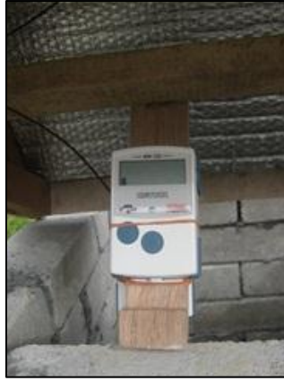
Figure 3.16: Position of hygro-thermometers inside house model (front view)
