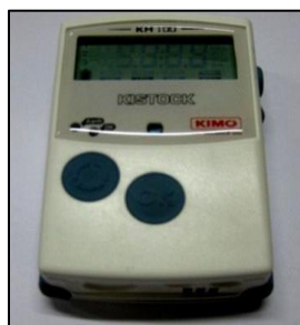
Figure 3.15: Hygro-thermometer with a built-in temperature and relative humidity sensor
