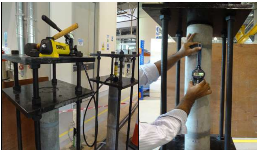
Figure 3.31 Creep Test Set up
