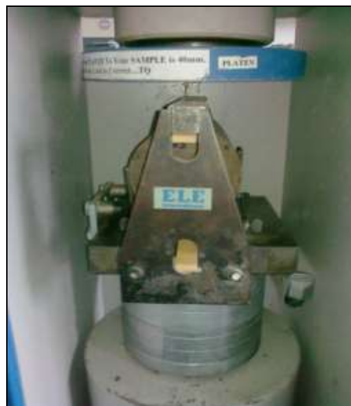
Figure 3.22 Splitting Tensile Strength Test
