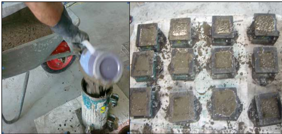
Figure 3.11 Casting of SCGC Mix Specimens
