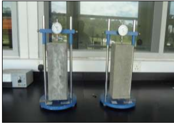
Figure 3.34 Drying Shrinkage Test Set up
