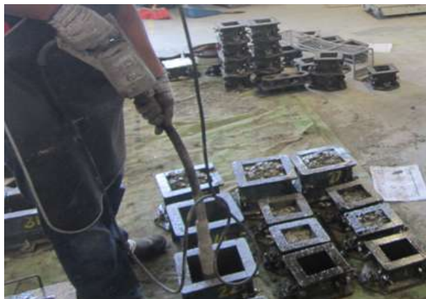
Figure 3.17 Casting of OPC Control Mix Specimens
