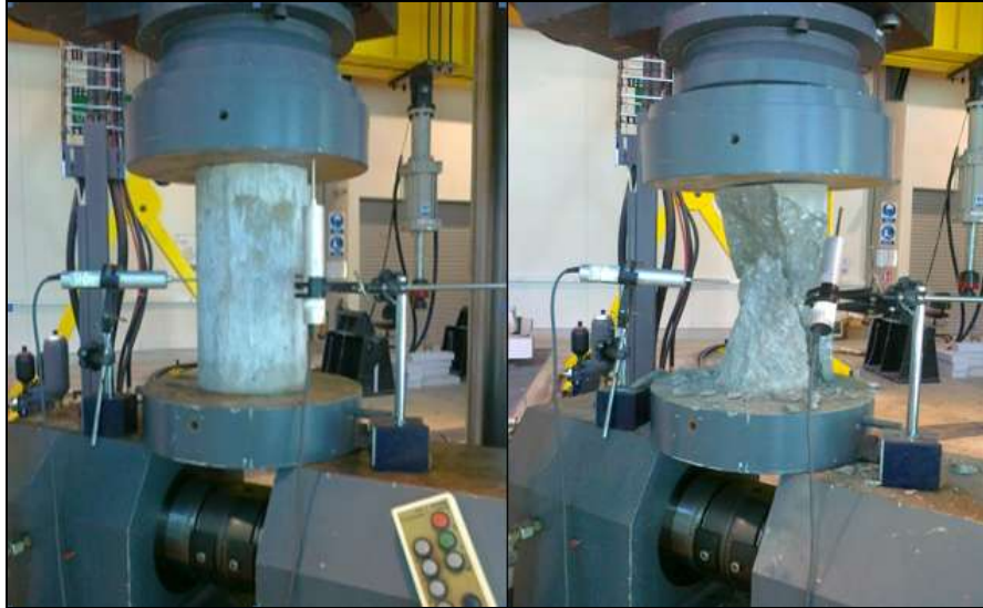
Figure 3.25 Modulus of Elasticity Test
