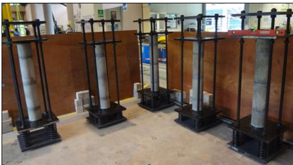
Figure 3.29 Creep Frames with Specimens
