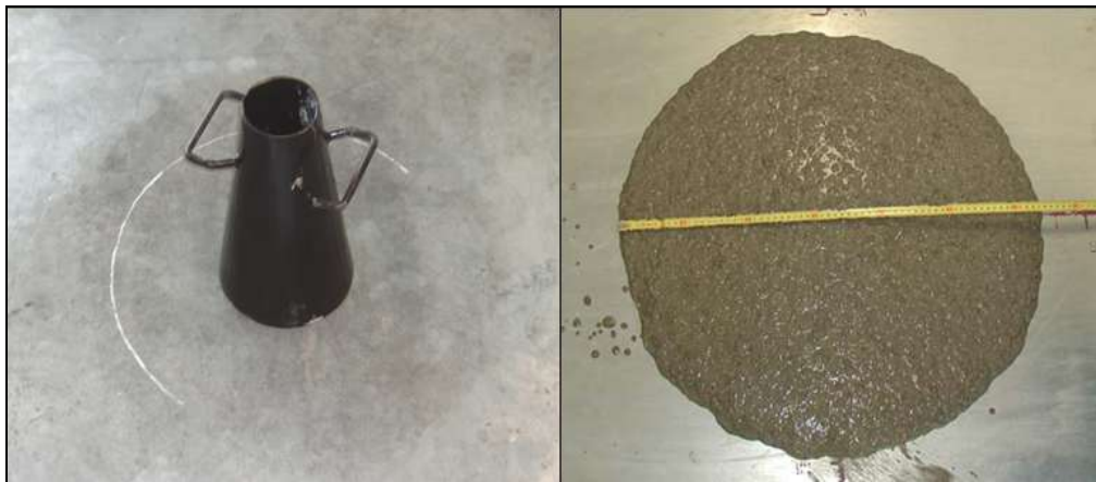
Figure 3.7 Slump Flow Test
