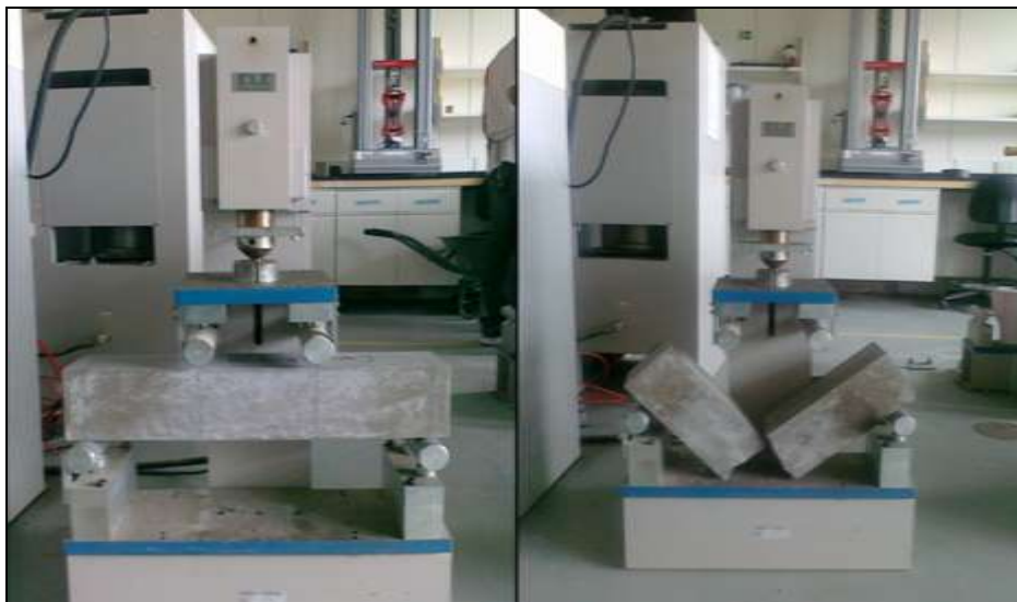
Figure 3.24 Flexural Strength Test
