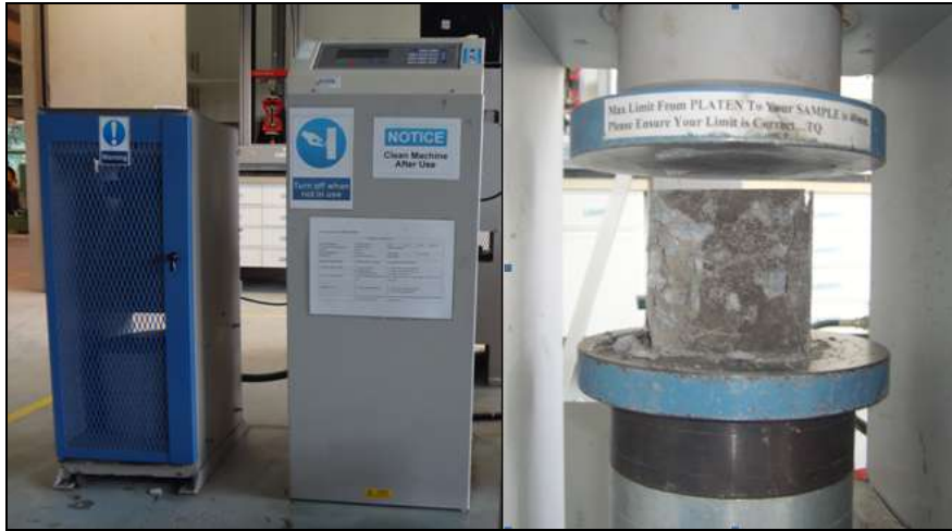
Figure 3.14 Compressive Strength Test
