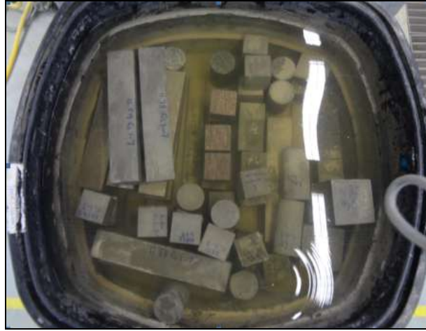
Figure 3.18 Curing of OPC Control Mix Specimens
