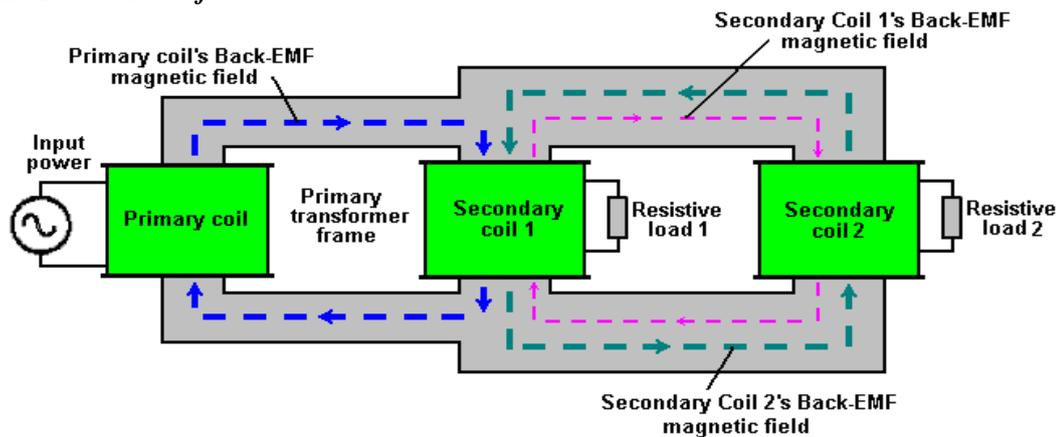
**Figure 2 Bi Toroid Transformer Pulse Movements**
