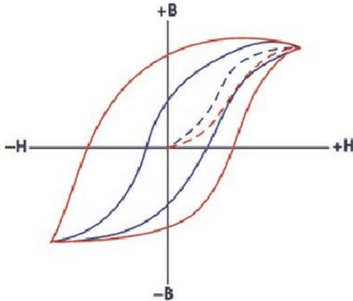
**Figure 8: Hysteresis Loop (Iron VS Permalloy)**
