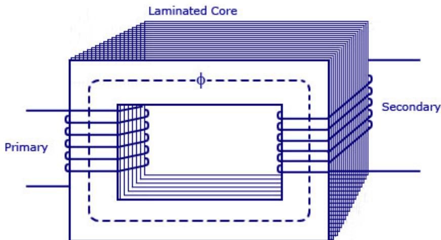
Figure 3 Conventional Transformer
