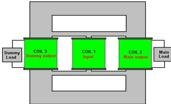
Figure 4 Bi Toroid Transformer
