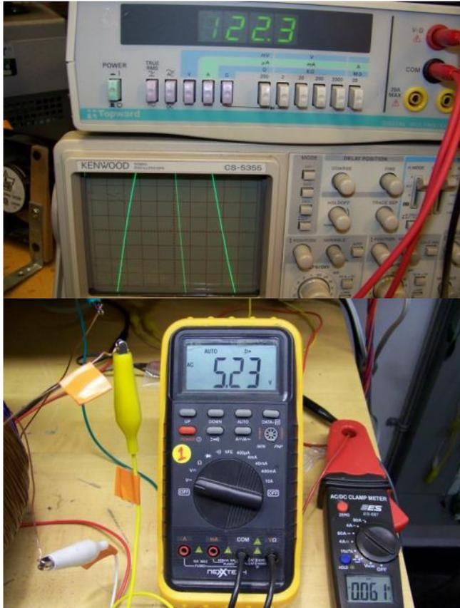
**Figure 14 Bi Toroid Transformer Efficiency Test**
