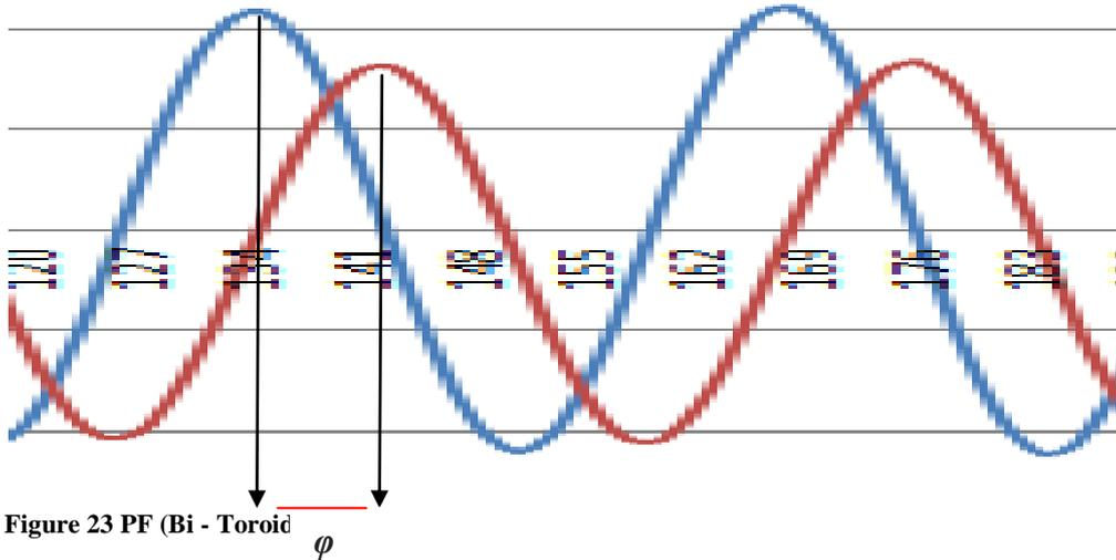
From the above graphs, it shows that the current and voltage for a Bi-Toroid transformer are almost  $90^\circ$  apart on the primary side. This means:
