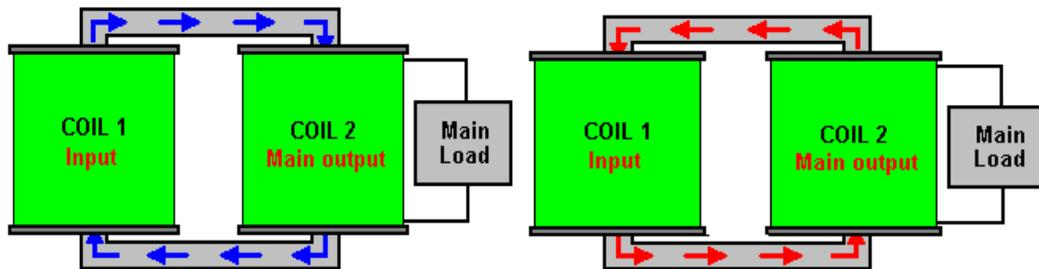
Figure 1 Conventional Transformer pulse movements
