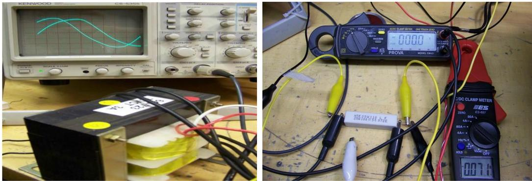
Figure 16 No Load Test
