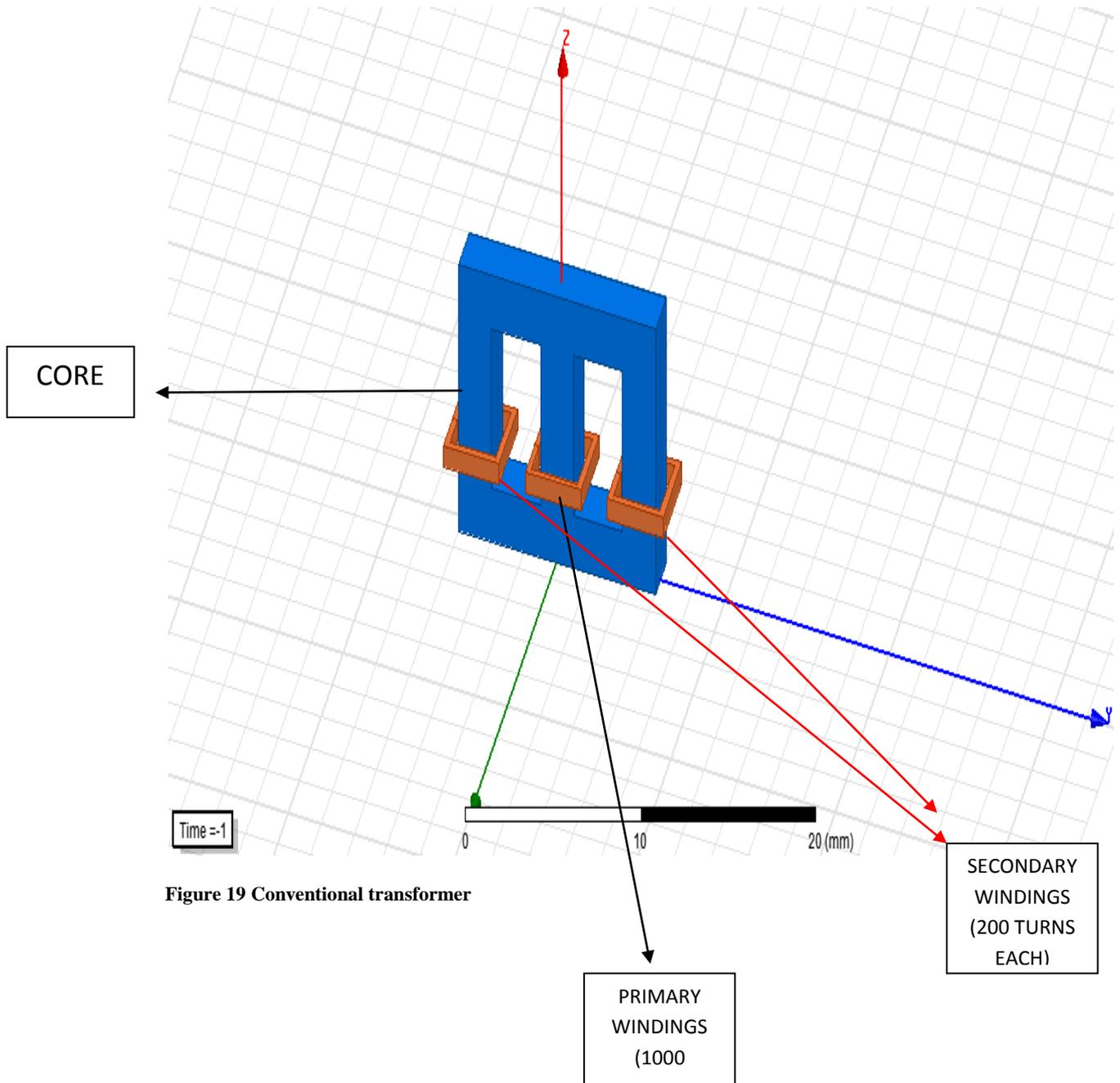
Figure 19 Conventional transformer
