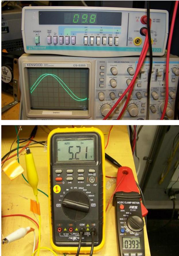
**Figure 13 Conventional Transformer Efficiency Test**
