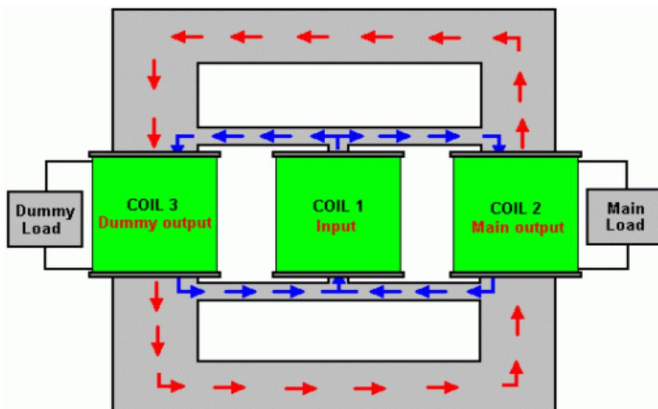
Figure 5 Bi Toroid Operating Principle
