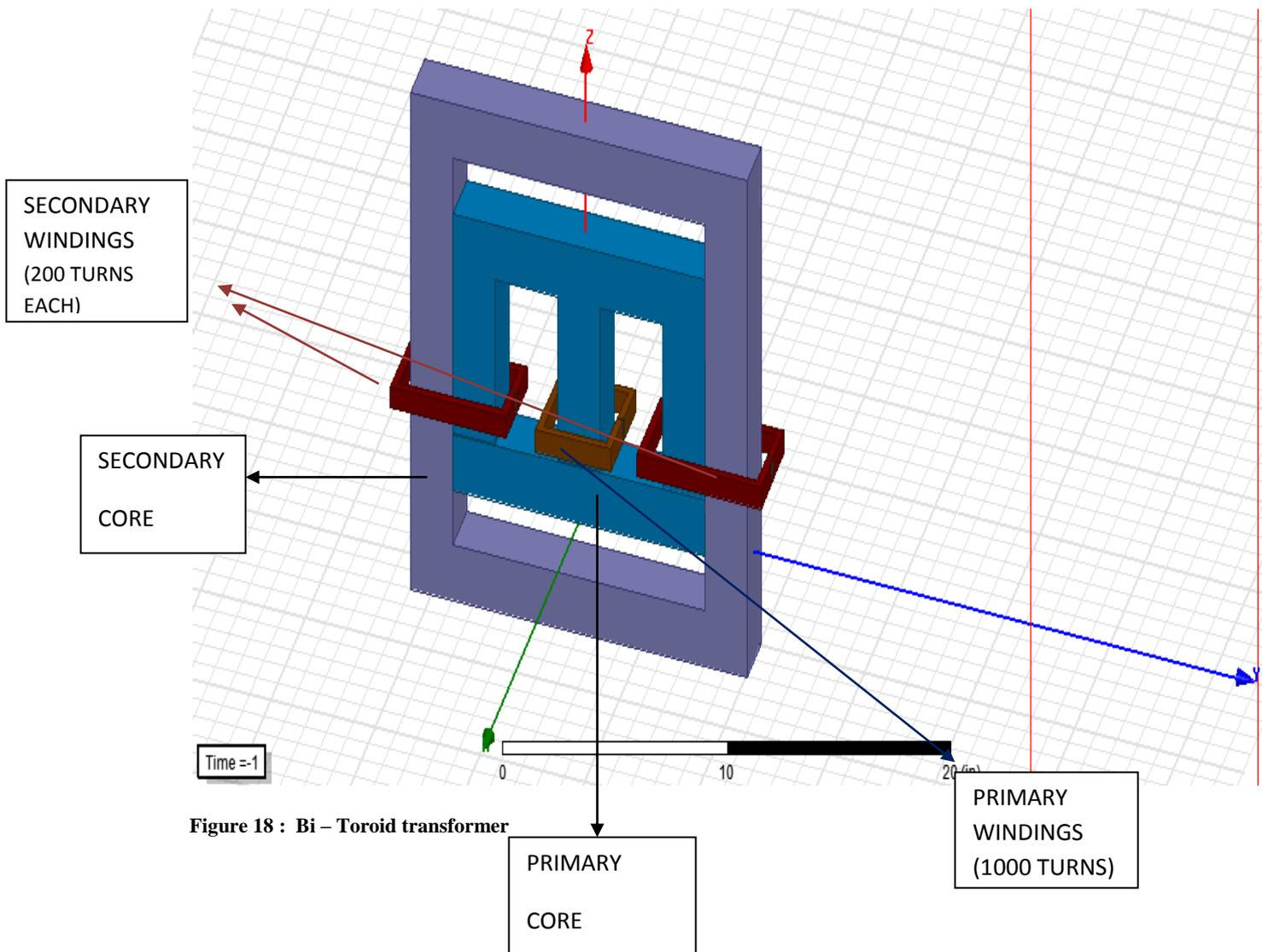
Figure 18 : Bi – Toroid transformer
