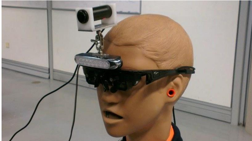
Figure 33: Smart Vein Locator
