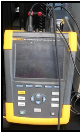
Figure 11: Fluke 435 three phase power quality analyzer
