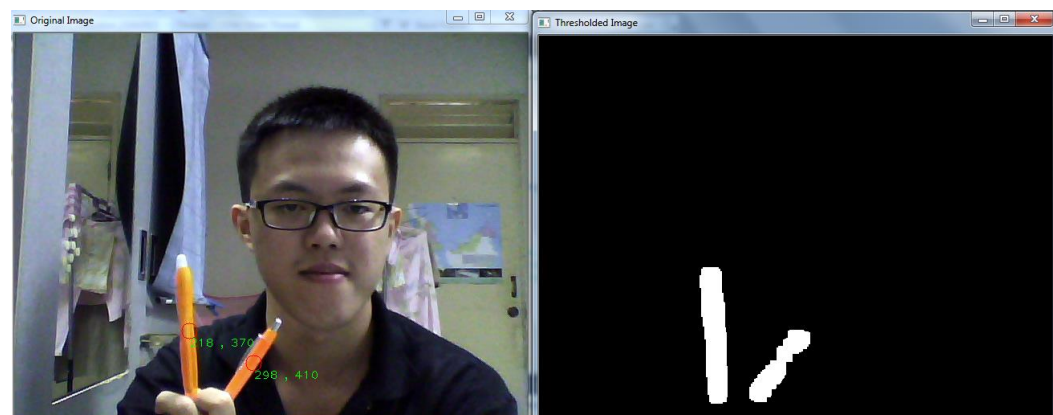
Figure (28) : Calibration for orange color to detect orange static obstacles. The value of HSV for orange: minimum HSV= (5,163,117), maximum HSV=( 23,231,256).
