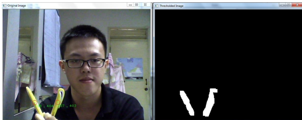
Figure (27) : Calibration for yellow color to detect yellow static obstacles. The value of HSV for yellow: minimum HSV= ( 26,81,153), maximum HSV=( 91,186,256).
