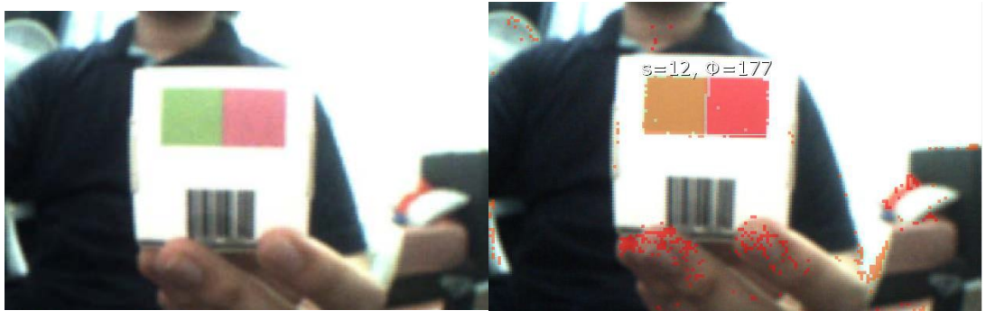
FIGURE 18: Pixy detecting colour codes with angle shown
