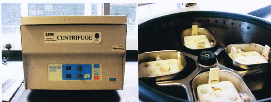
Figure 3.5: Centrifugal Separator
