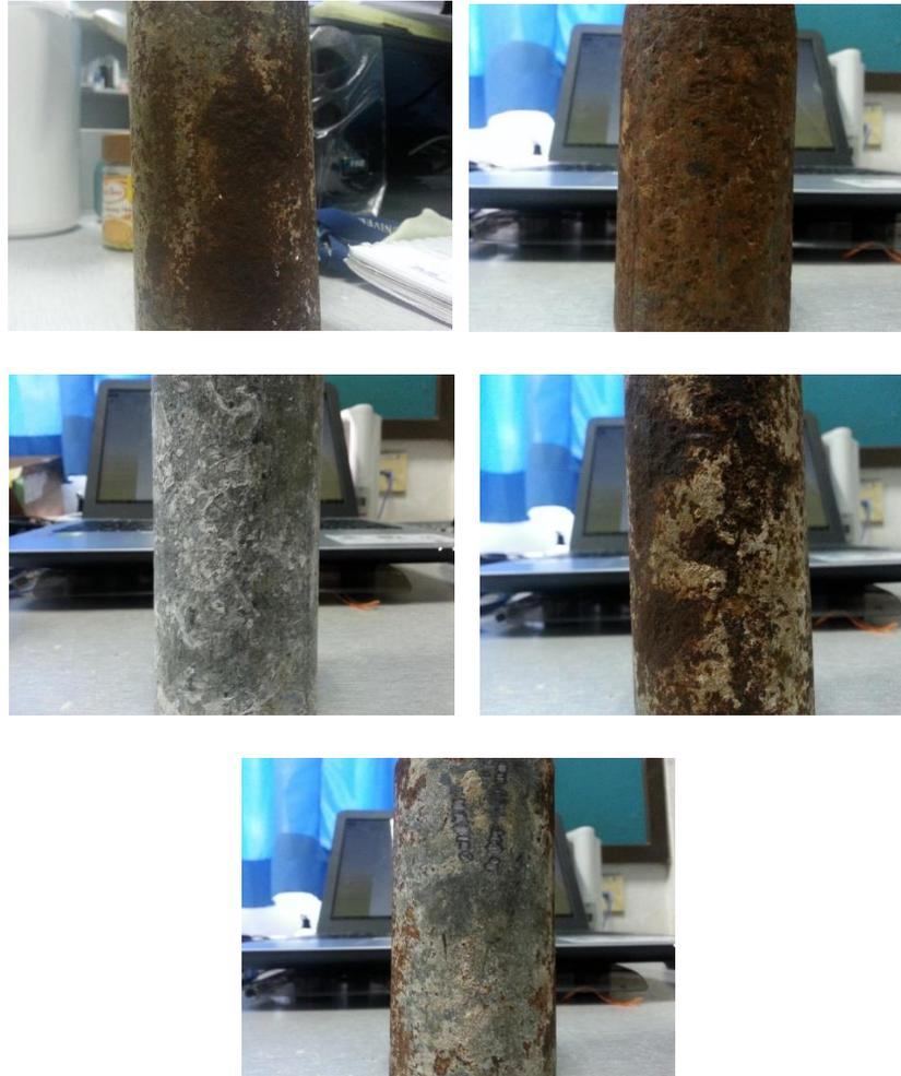
Figure 2. Samples with different degree of corrosion
