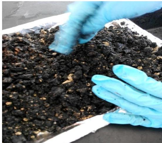
FIGURE 3.4 Mix of Petroleum Sludge with Additives
