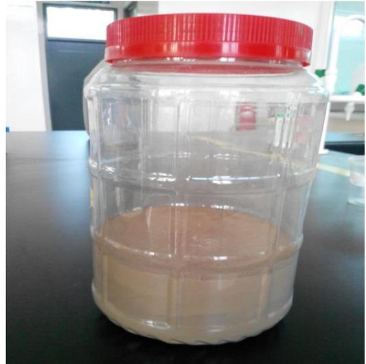
FIGURE 3.7 Residue Ash after Grinded
