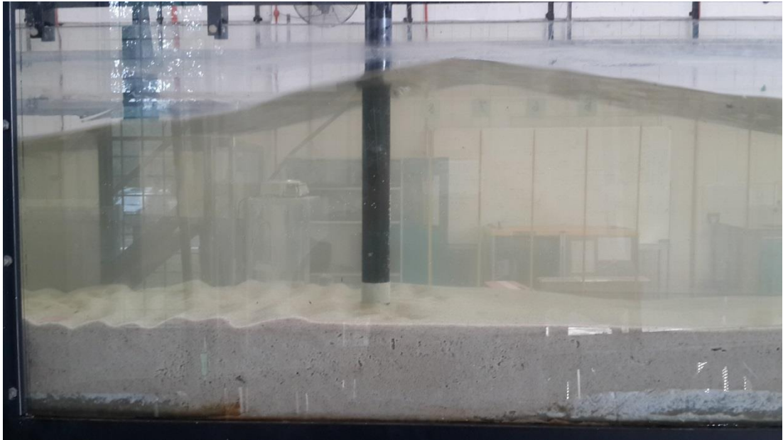
Scour Formation during Experiment
