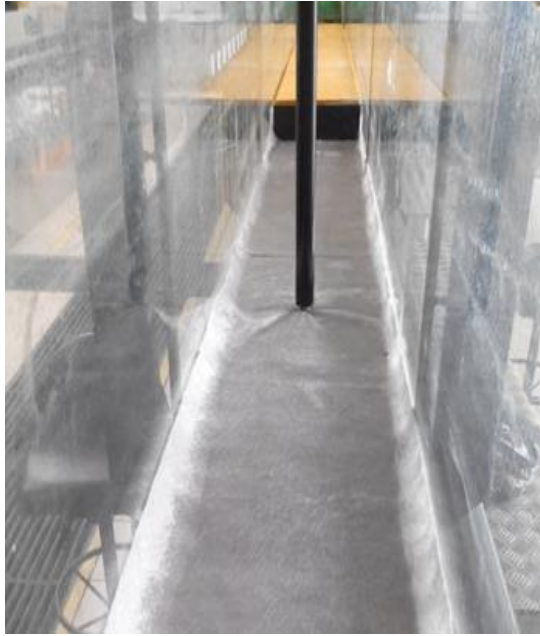
Figure 3-10: Underlying Geo Textile On Bed Of Flume
