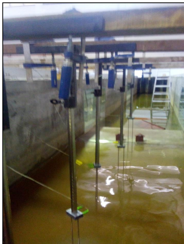
Figure 4.7 : Position of Wave Gauge Probe
