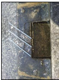
Figure 12: Deflectors at an angle of 45^{\circ} which produced the highest efficiency.
