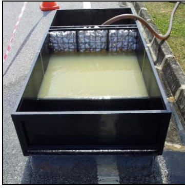
Figure 11: Collection tank used to produce sheet flow
