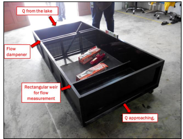
Figure 10: Plan view of collection tank for field investigation
