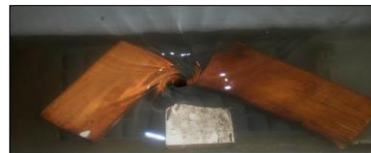
Figure 5: Orifice flow through a grate inlet
