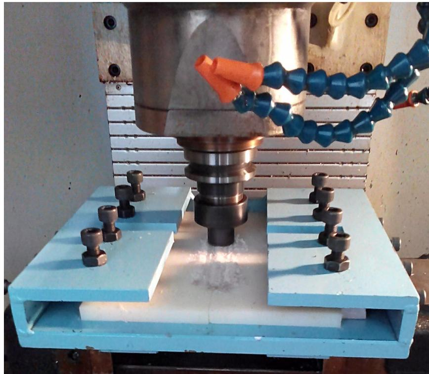
*Figure 12 FSW with the presence of blue Nylon 6 Markers*
