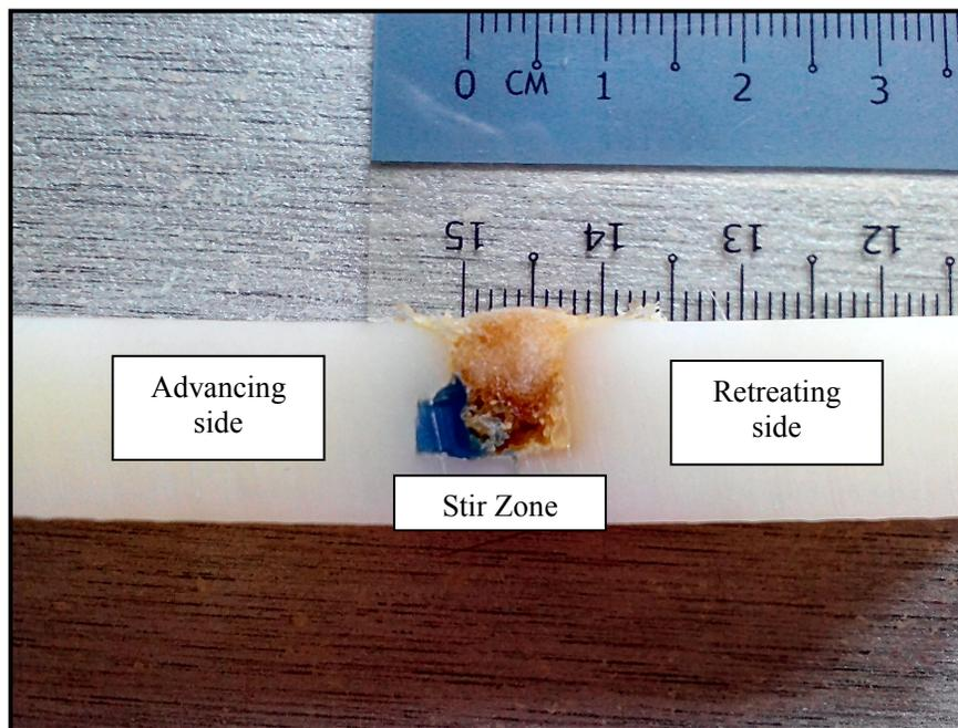
*Figure 28 Cross-section of the butt weld joint at 40 mm/min*
