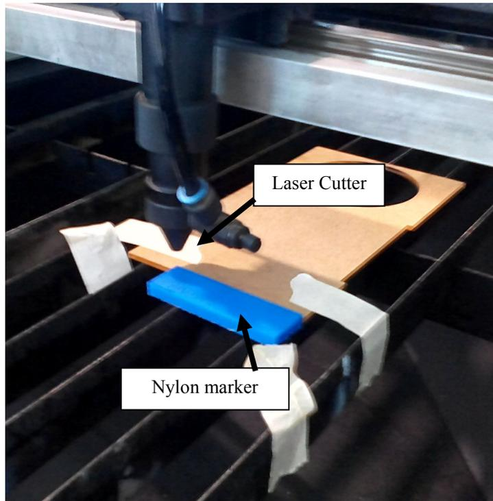
*Figure 11 Laser Cutter Machine slicing the blue-coloured Nylon material*
