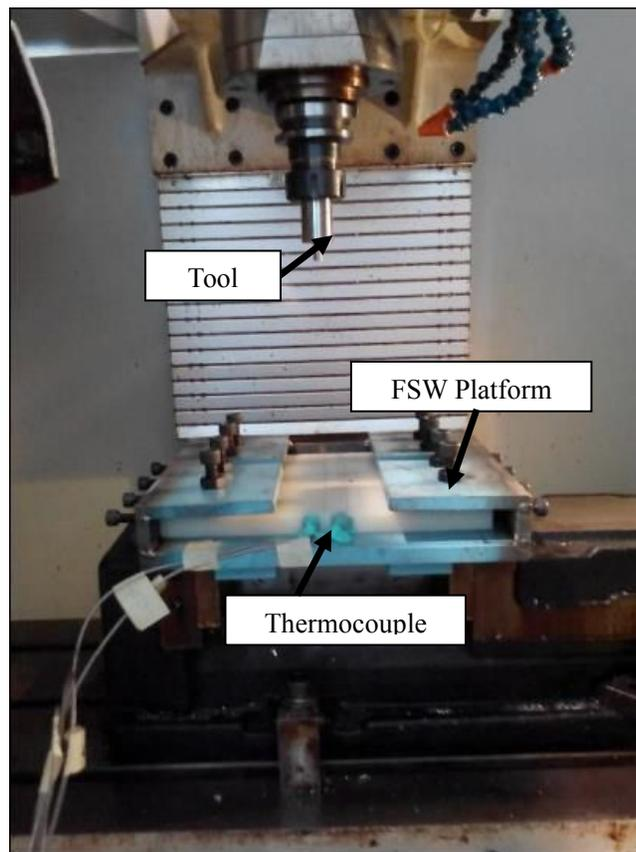
*Figure 8 Experimental Setup of FSW on Nylon 6 Plates*
