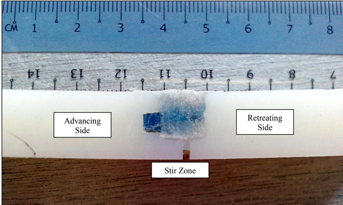
**Figure 22** Cross-section of the butt weld joint at 25 mm/min
