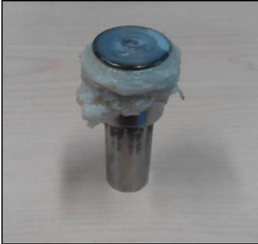
*Figure 15 Pin Profile with breakage*
