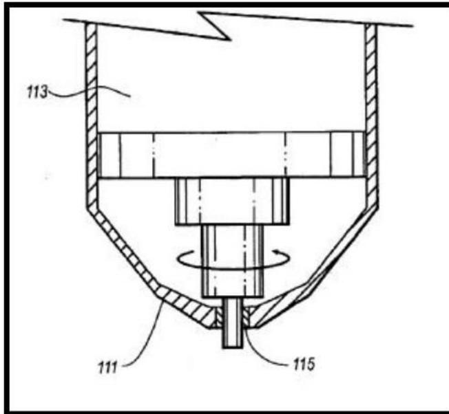
Figure 32 A schematic of a comparative spindle shoulder
