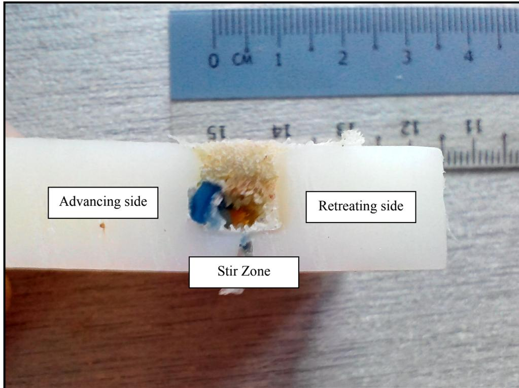
**Figure 26** Cross-section of the butt weld joint at 35 mm/min
