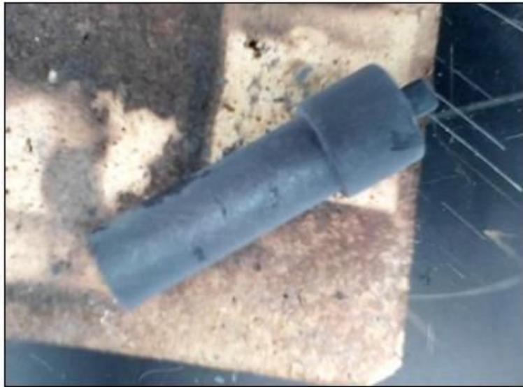
*Figure 7 Fabricated Tool after Heat Treatment*
