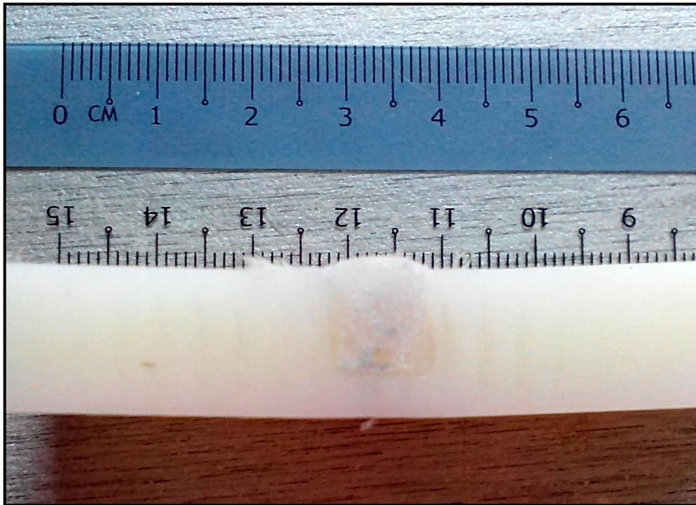
**Figure 29** *Cross-section of the butt weld joint at 30 mm/min without markers*
