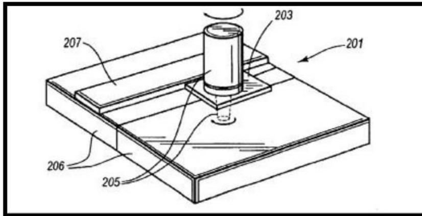
Figure 33 Constrained surface is the form of hot tool shoe
