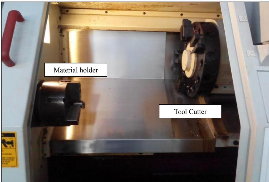
*Figure 3 Utilizing CNC Lathe Machine for tool fabrication*
