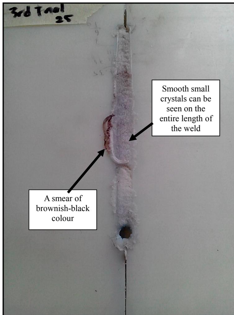
*Figure 21 Appearance of Nylon 6 Plates Welded at 25 mm/min*
