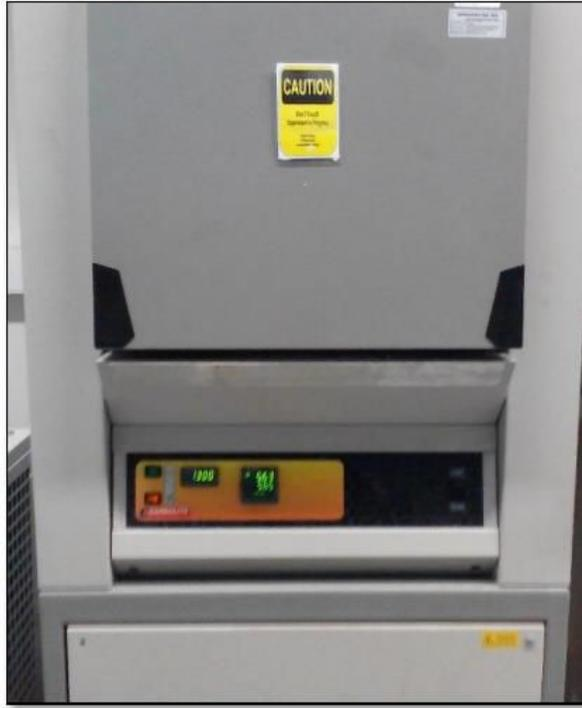
*Figure 6 Furnace Unit for Heat Treatment Process*
