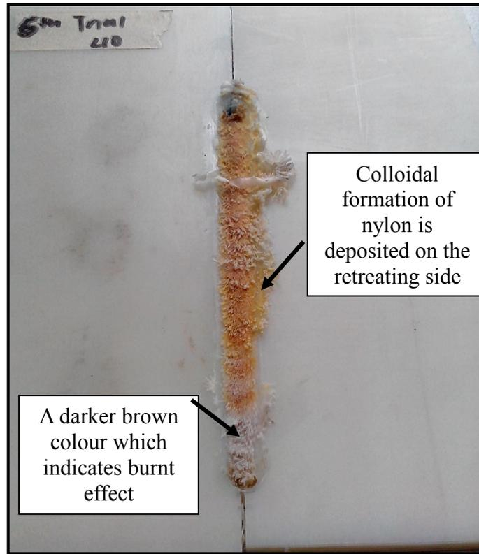
*Figure 27 Appearance on Nylon 6 Plates at feed rate of 40 mm/min*
