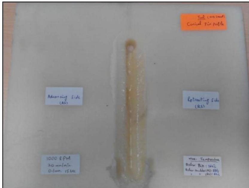
*Figure 17 FSW with Conical Pin Profile*
