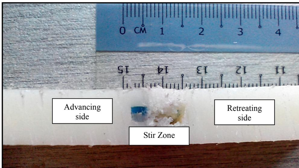
*Figure 24 Cross-section of the butt weld joint at 30 mm/min*
