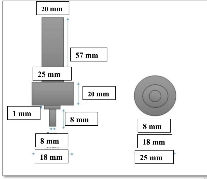
*Figure 1 Tool geometry with two shoulders and a cylindrical pin profile*
