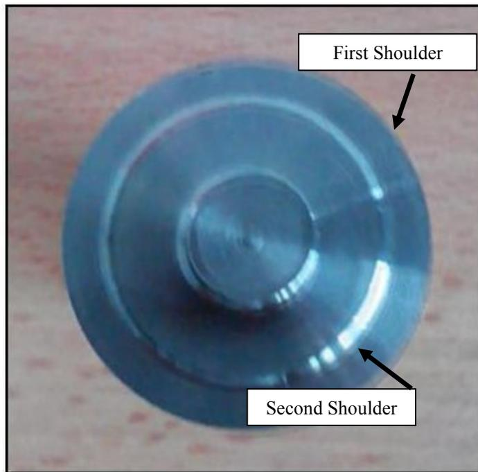
*Figure 5 Fabricated Tool Top View*
