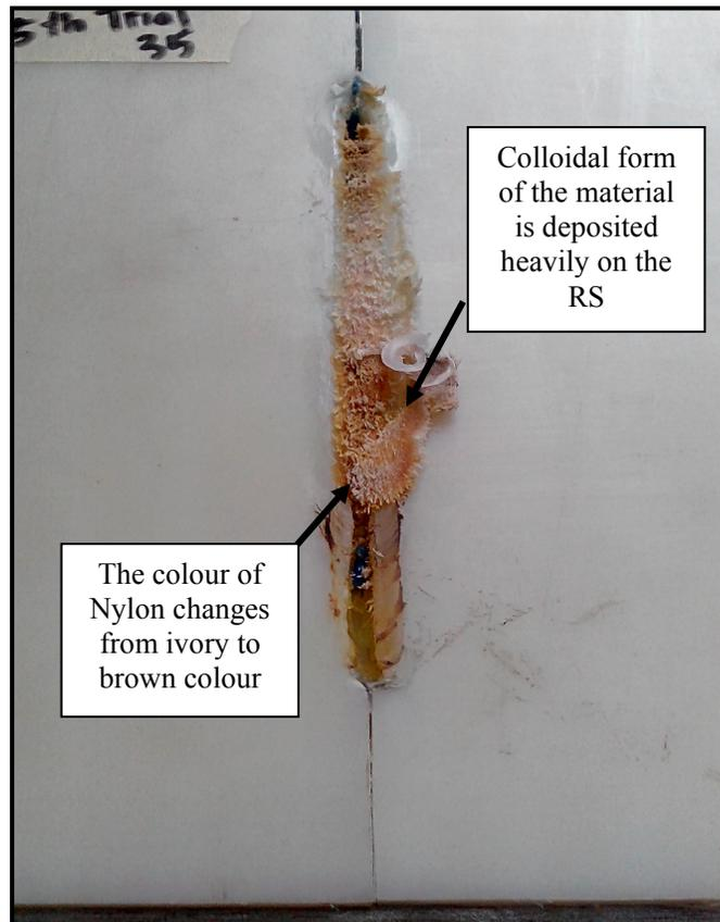
**Figure 25** Appearance on Nylon 6 Plates at feed rate of 35 mm/min
