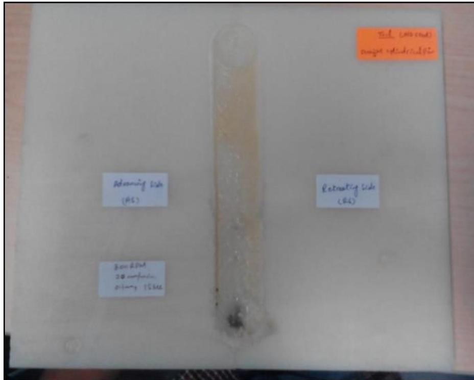
*Figure 14 FSW with Straight Cylindrical Pin Profile*
