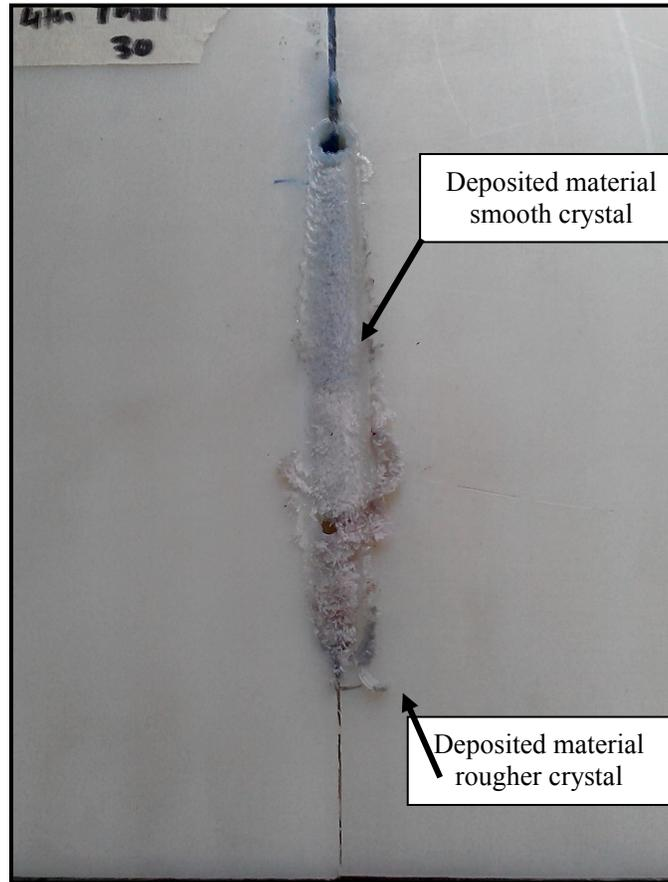
*Figure 23 Appearance on Nylon 6 Plates at feed rate of 30 mm/min*
