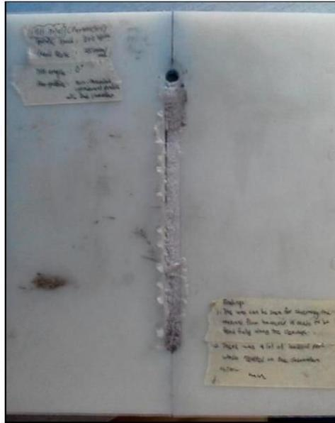
**Figure 19** First Trial of The FSW with Paraffin Wax Marker
