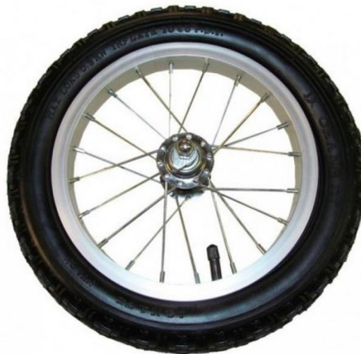
Figure 2.19: Allow wheel with pneumatic tire (Ed Grabianowski, 2007)
