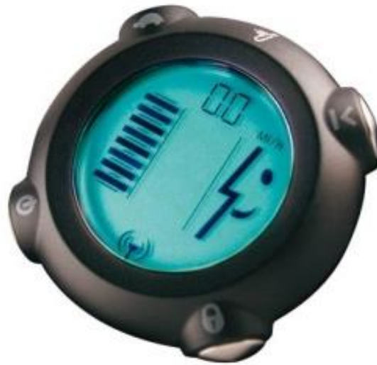
Figure 2.23: A smile face shown means Segway is ready to ride and vice versa ("Safety In Design | Segway Safety," 2010)
