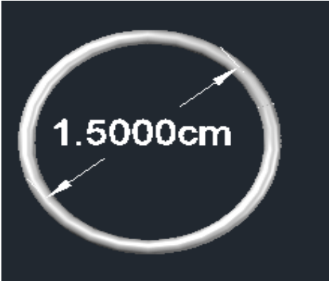
Figure 4-5: Final Design of Induction Coils A4 (Front View)
