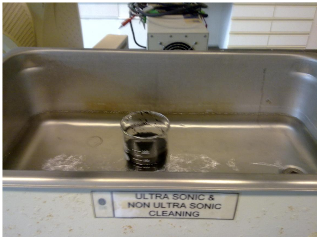
Sonication Process of CNT in de-ionized water
