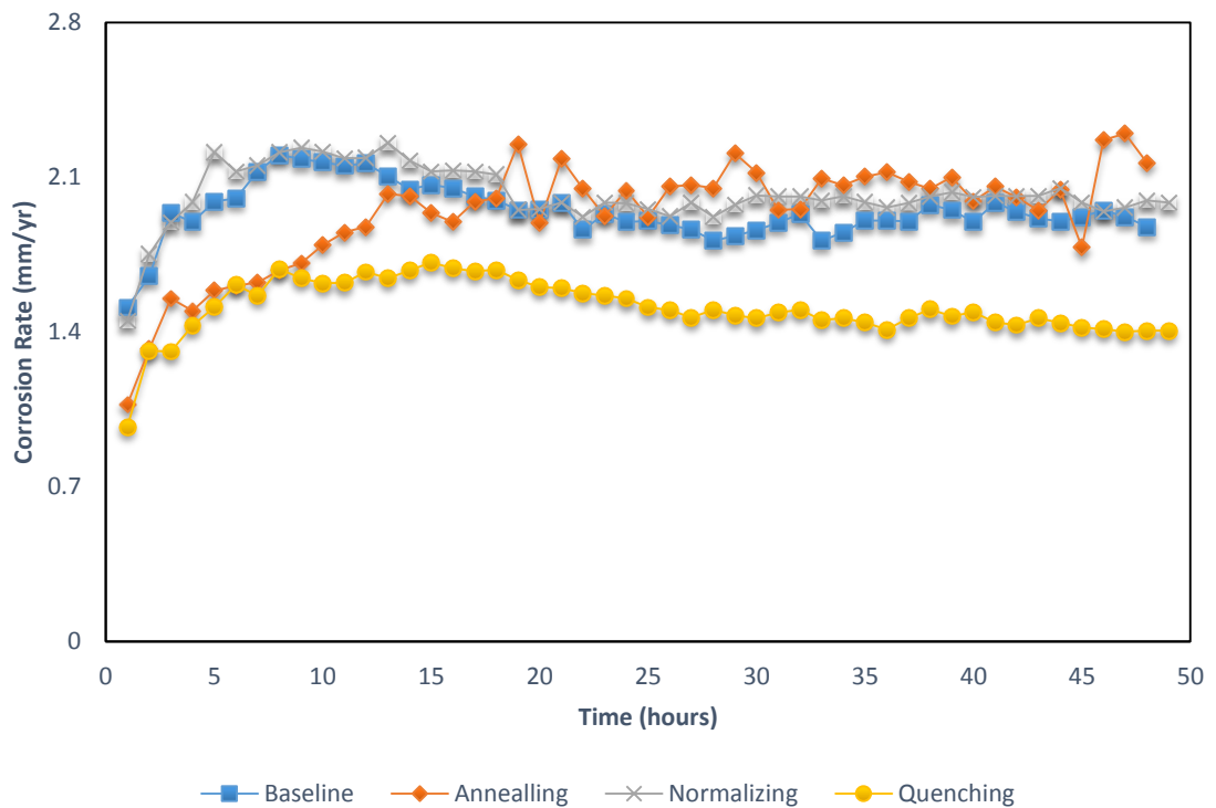
Figure 18: LPR Corrosion Rate against Time with Presence of Acetic Acid (1000ppm)
