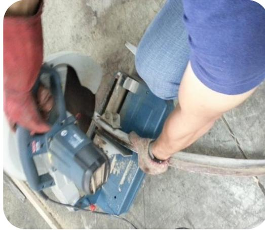
Figure 3.7 Cutting feedstock using power saw
