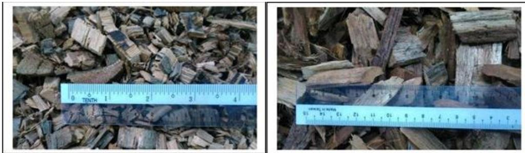
Figure 3.8 Size of feedstock after cutting Cocont frond (left) and wood (right)
