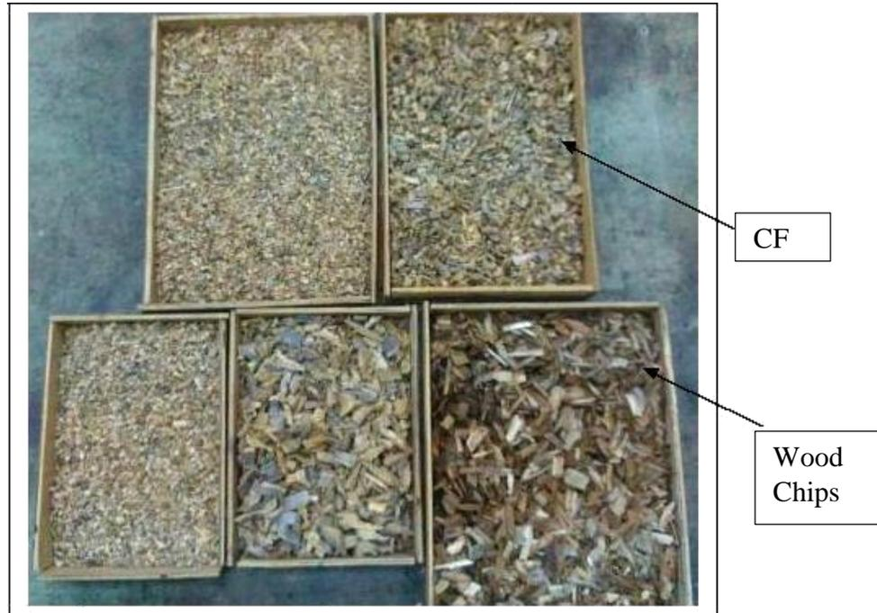
Figure 3.10 Raw CF and Wood Chips before mixing
